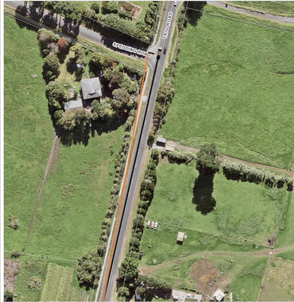
Figure 2: Sight distance south at the Trig Rd / Spedding Rd intersection (sight distance calculation lines in black, vegetation clearance extent between black and orange lines)
