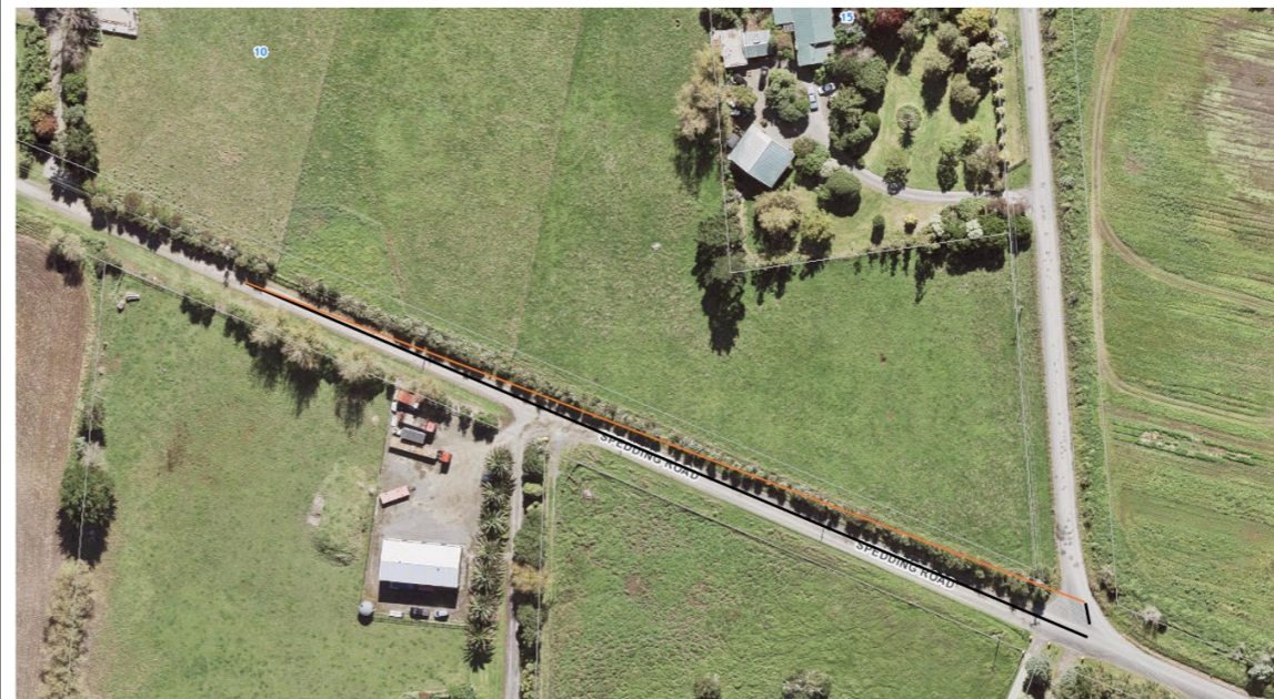
Figure 3: Sight distance west at the Spedding Rd / Mamari Rd intersection (sight distance calculation lines in black, vegetation clearance extent between black and orange lines)
