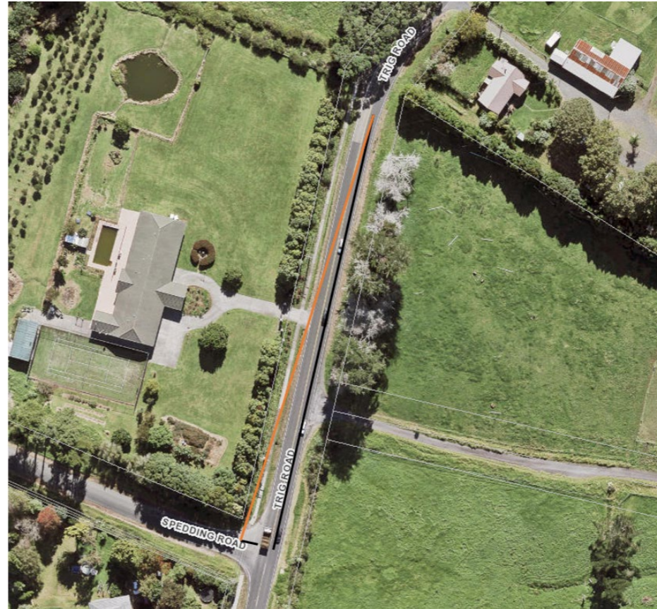
Figure 1: Sight distance north at the Trig Rd / Spedding Rd intersection (sight distance calculation lines in black, vegetation clearance extent between black and orange lines)
