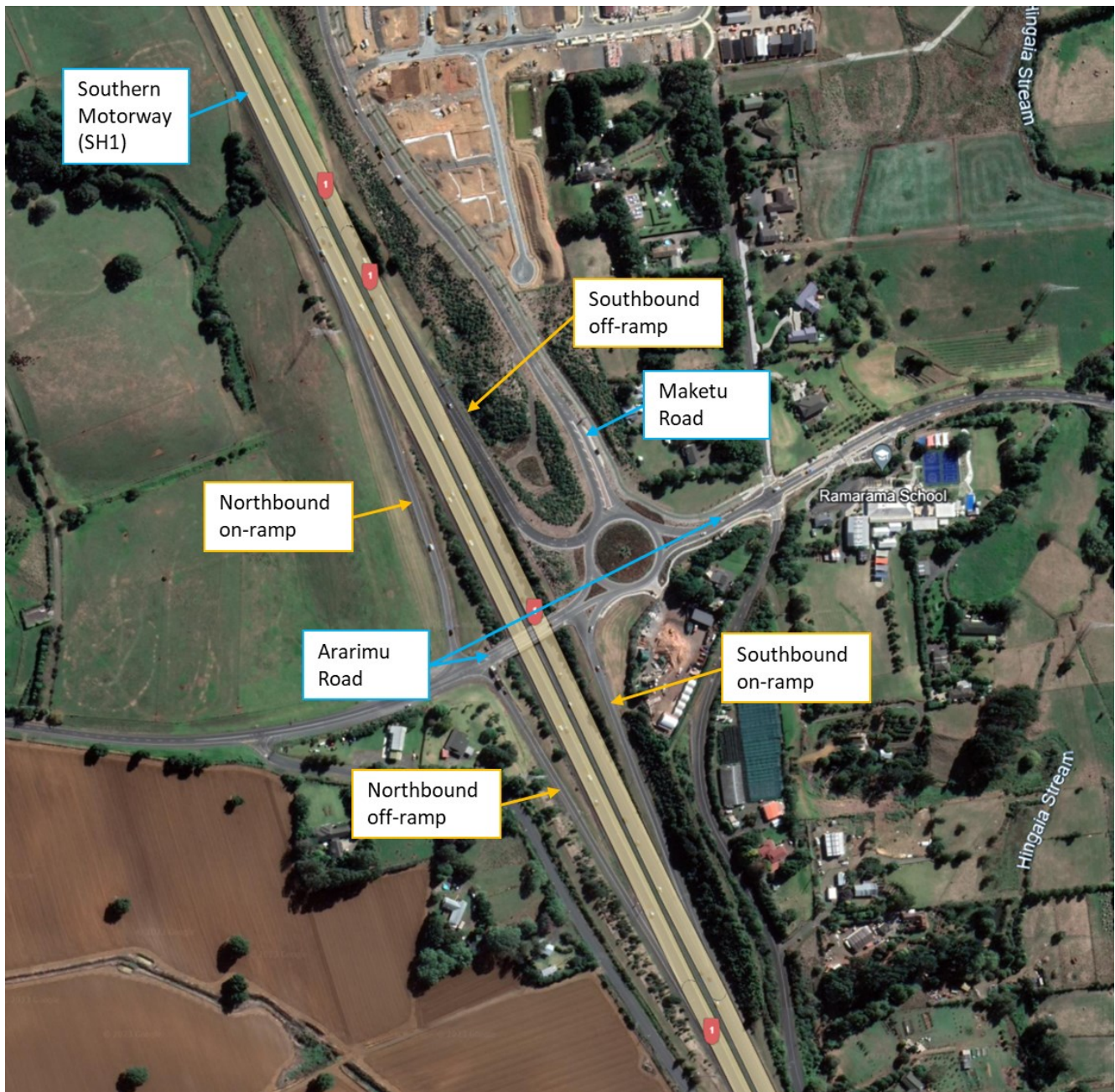
Figure 5-4: Existing Layout at Ramarama Interchange
