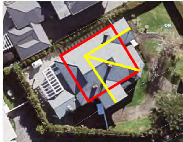
Figure 96: 120 Hinemoa Street, showing the more common arrangement of bays in a corner bay villa (yellow) over the basic form of the house (red) (Auckland Council GeoMaps)
