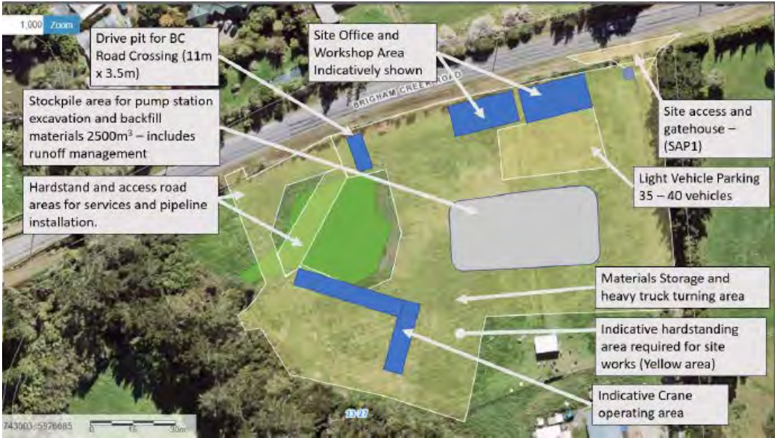
Plate 3. Proposed Contractor Area Layout (Approx.)
