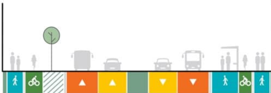
Figure 3: Indicative Fred Taylor Drive Cross Section
