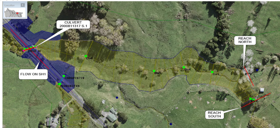
Figure B:8.7.b Model results over the SH1 over 2000mm \phi x2 culvert
