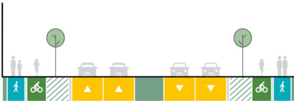
Figure 1-5: Indicative Cross Section Brigham Creek Road between Totara Road and Tamatea Road
