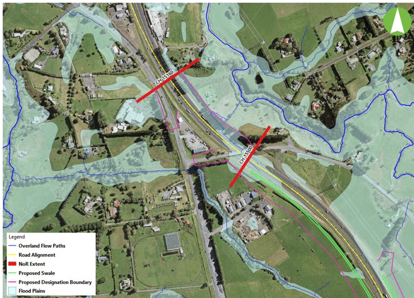
Figure 6-3 Proposed swale within NoR 1 project boundary
