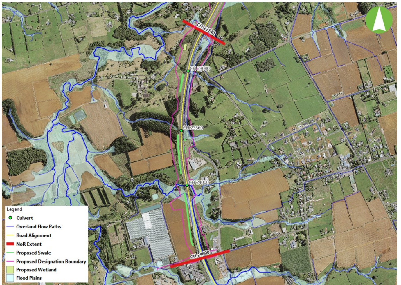
Figure 8-3 Proposed swale locations within NoR 3 project boundary
