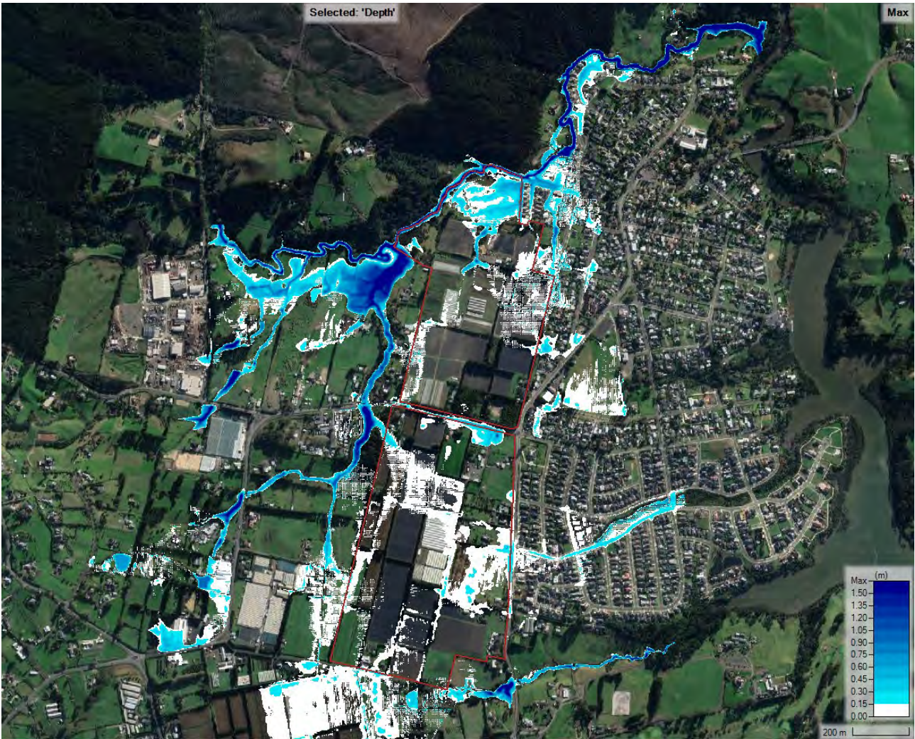
Figure 22: Maximum Flood Depth Map for Pre-development(SiteED+External ED) for combination of 2yr+100yr without CC
