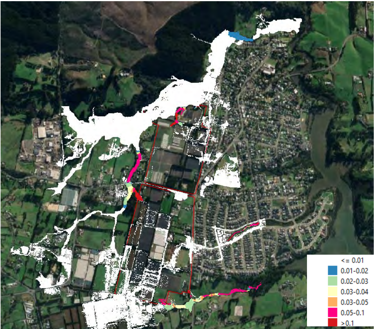
Figure 32: WSE Difference Map between Post-(SiteMPD+ExternalMPD) and Pre-development(SiteED+ExternalMPD) scenarios for 100yr + Climate Change 3.8°C
