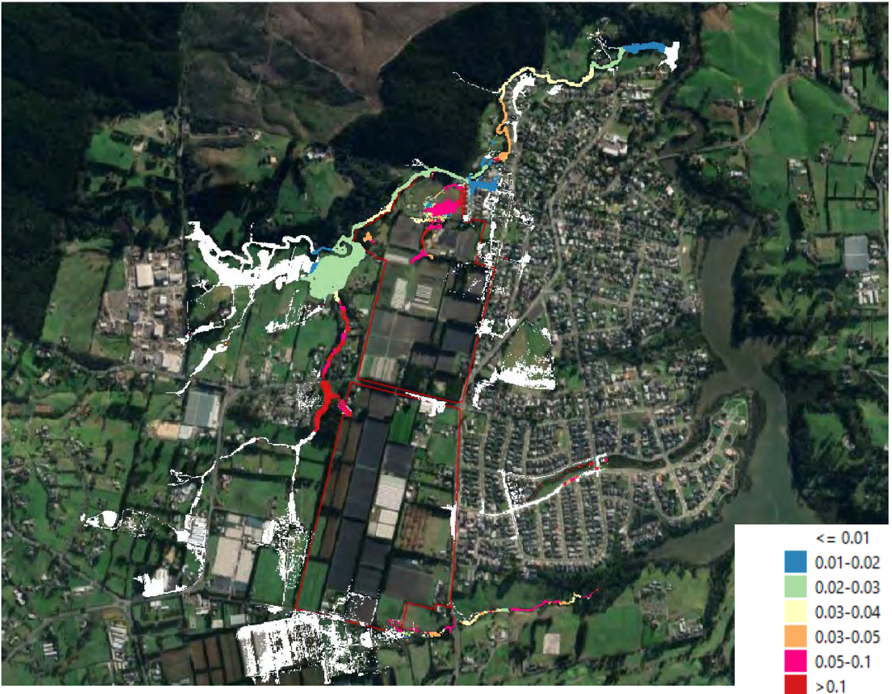
Figure 15: WSE Difference Map between Post-(SiteMPD+External ED) and Pre-development (Site ED+External ED) scenarios for 2yr without CC
