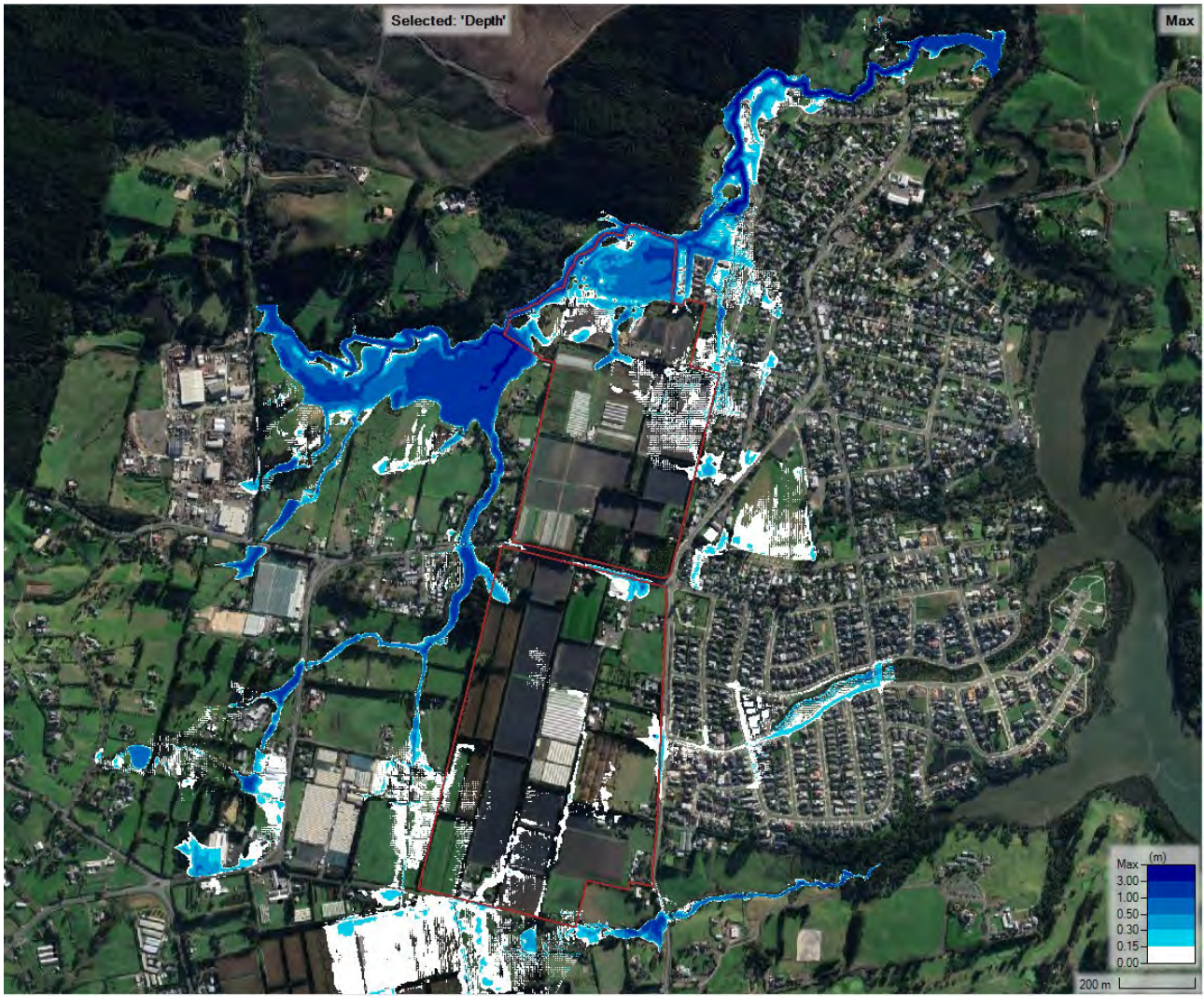
Figure 20: Maximum Flood Depth Map for Post-development (SiteMPD+External ED) for 100yr without CC
