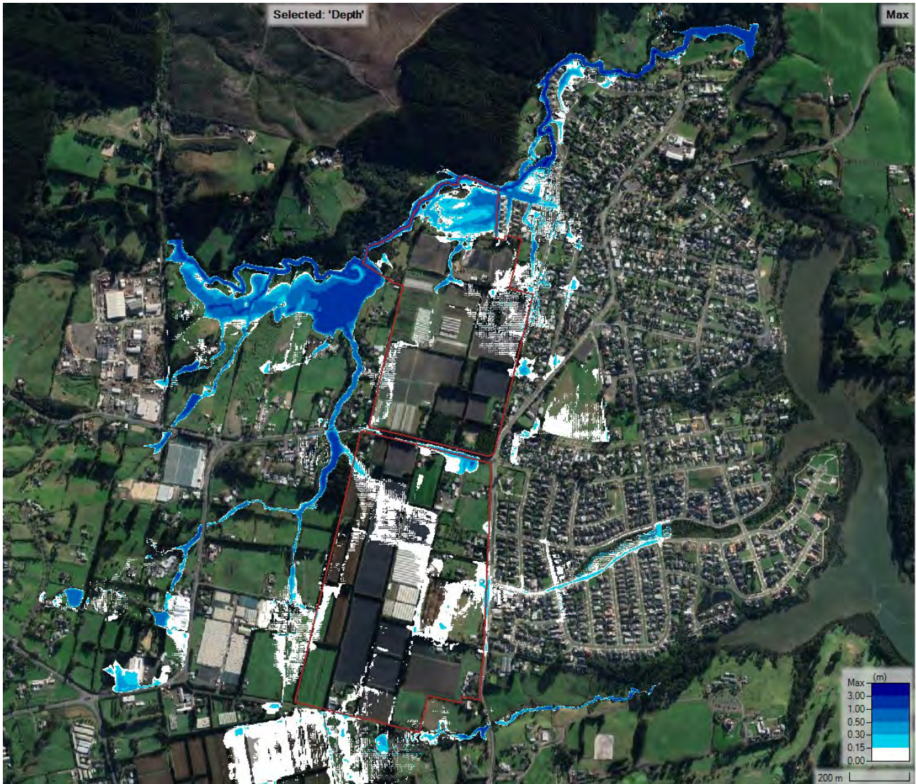
Figure 16: Maximum Flood Depth Map for Pre-development(Site ED+External ED) for 10yr without CC
