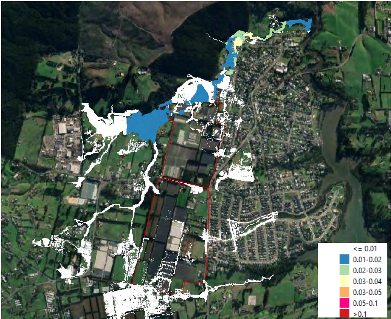
Figure 25: WSE Difference Map Between Attenuation Scenario and Post-development((SiteMPD+External ED) scenarios for 100yr without CC
