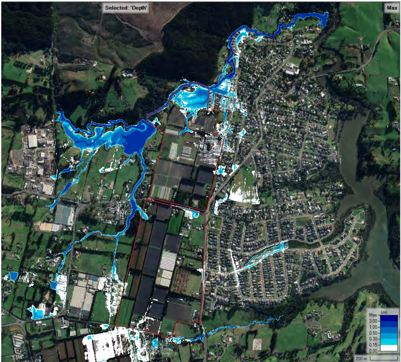
Figure 17: Maximum Flood Depth Map for Post-development (SiteMPD+External ED) for 10yr without CC
