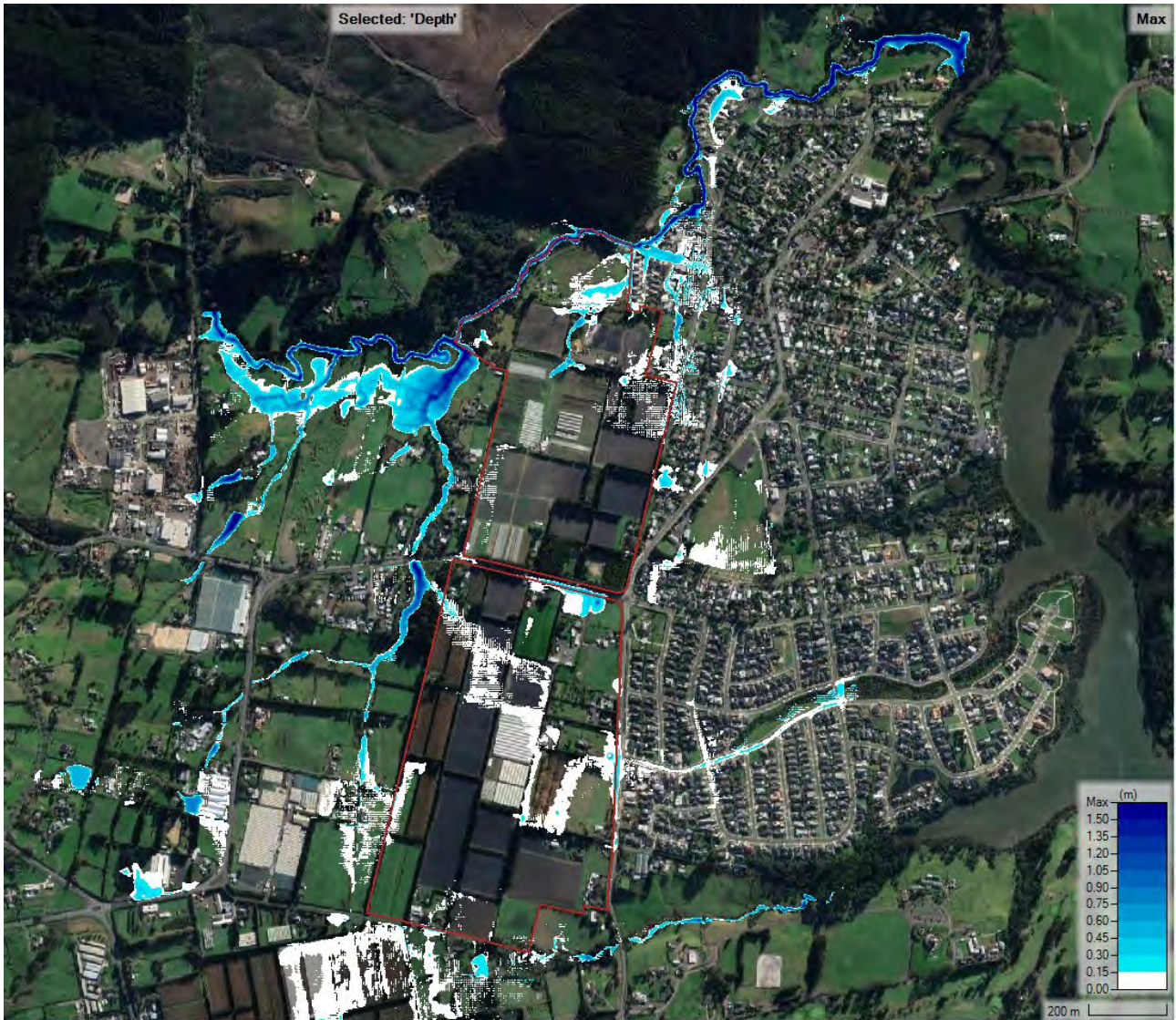
Figure 13: Maximum Flood Depth Map for Pre-development (Site and External ED) for 2yr without CC
