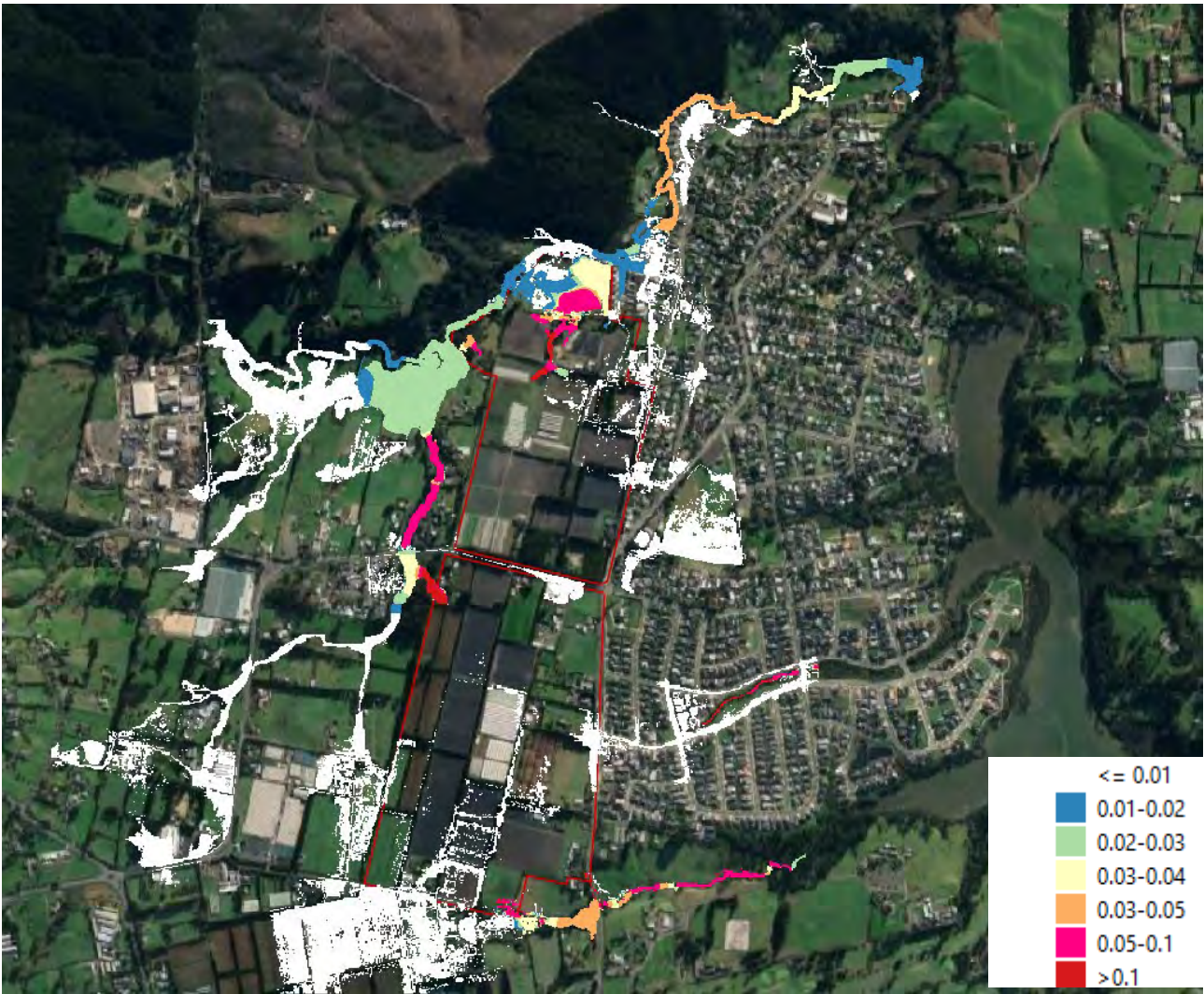
Figure 24: WSE Difference Map BETWEEN POST-development and Pre-development for Localized Impact Scenario (Combination of 2yr and 100yr without CC)
