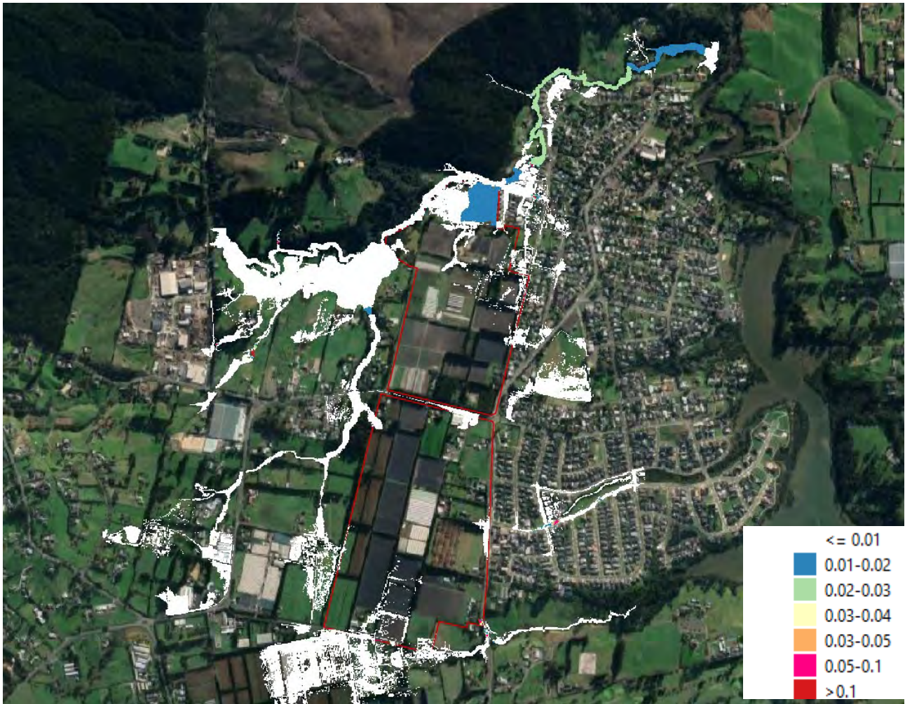
Figure 26: WSE Difference Map Between Post-development (SiteMPD+ExternalED) without Attenuation and With Attenuation On Site For 10yr without CC
