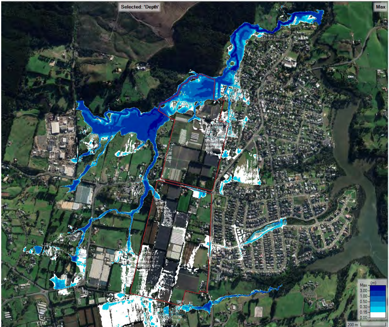
Figure 28: Maximum Flood Depth Map for Post-development (SiteMPD+External MPD) for 100yr + Climate Change 2.1°C
