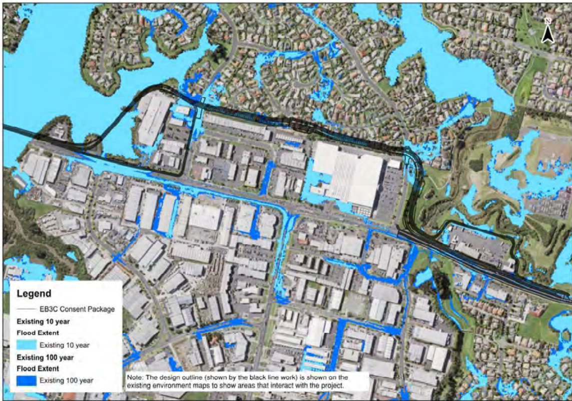
Figure 15. EB3C base case 10 and 100-year flood extents
