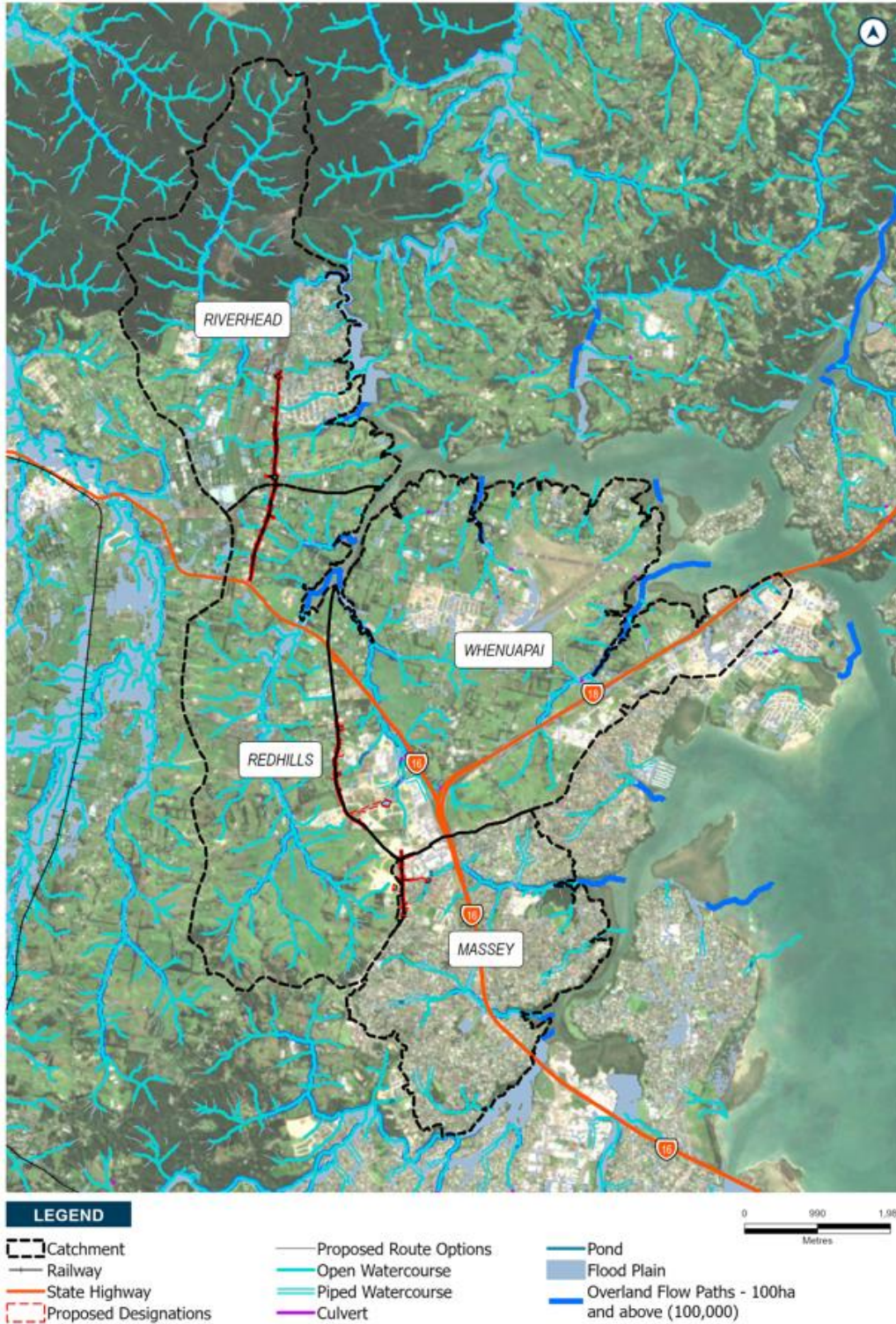
Figure 3-1: Existing 100 year ARI flood plain for Whenuapai, Massey, Riverhead and Redhills catchments (Auckland Council GIS)
