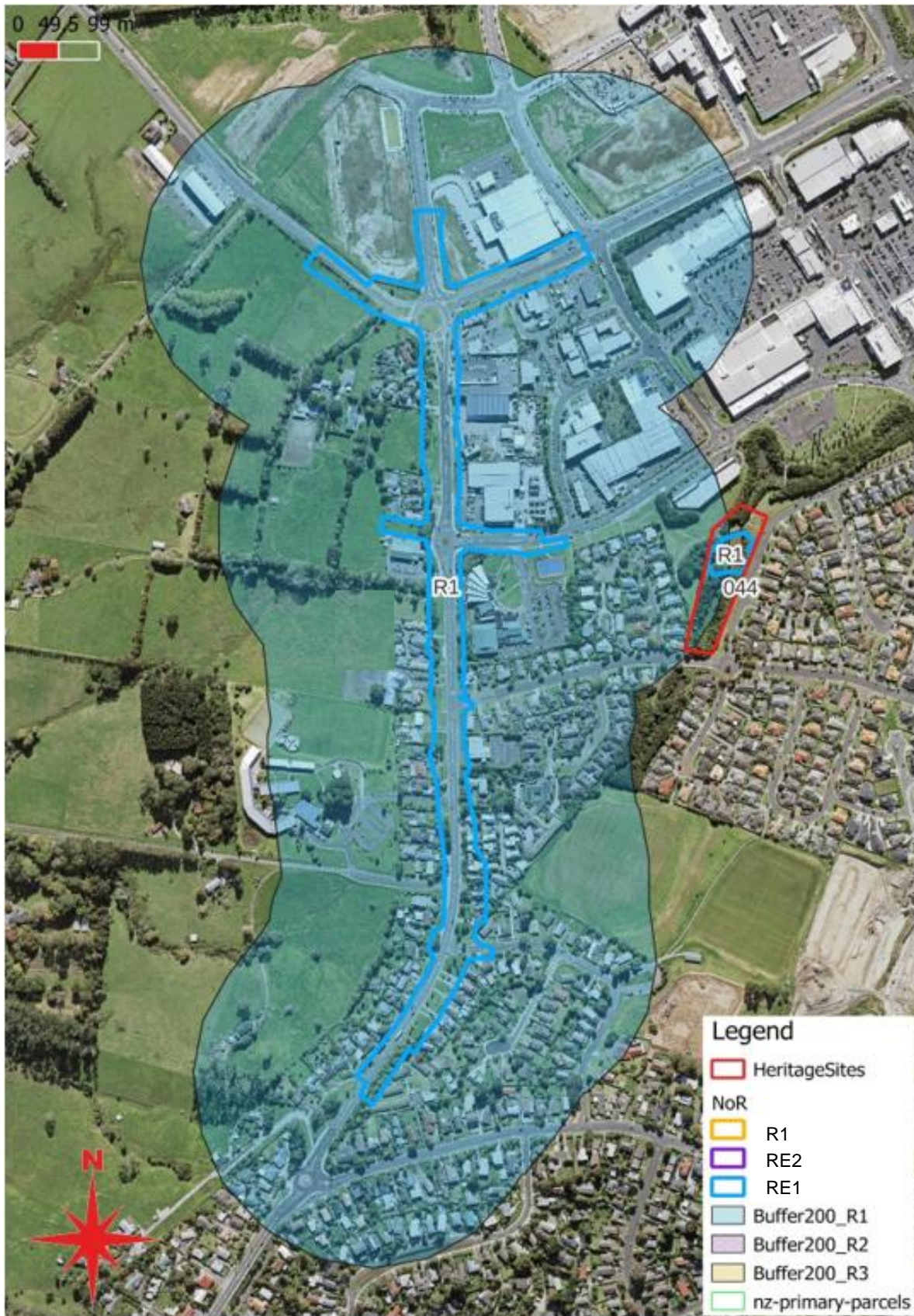
Figure 6-2: NoR RE1. The risk area around the stream is shown as 044. The picture also shows the 200 m buffer zone around the NoR of the road.
