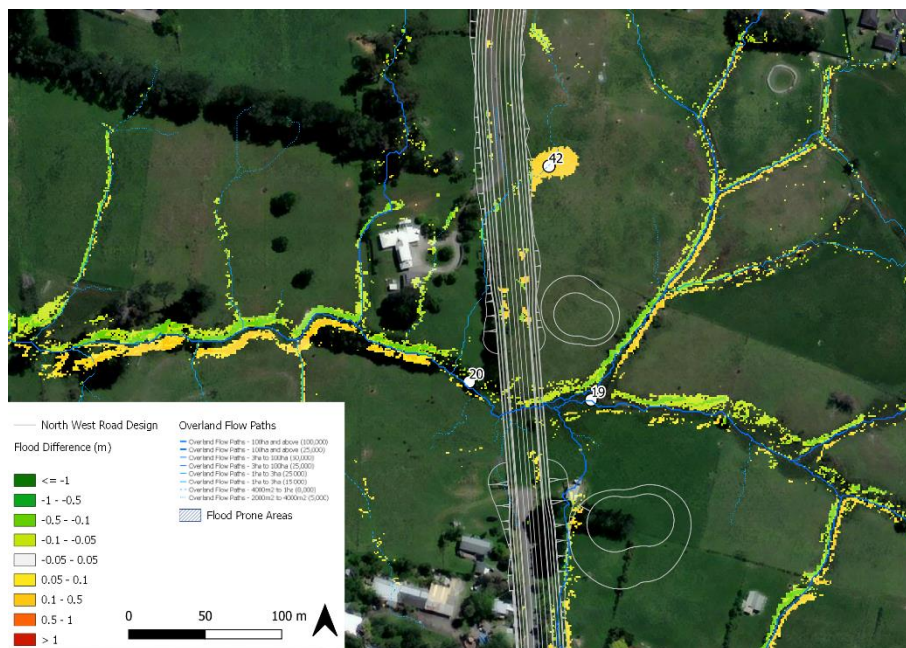
Figure 10-1: 100year flood difference map for Māmari Road (North) and Sinton Stream bridge crossing
