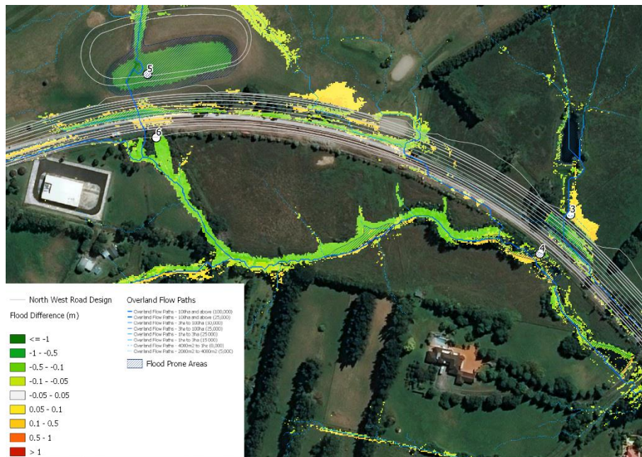
Figure 11-2: 100year flood difference map for Brigham Creek Road East of Trig Road
