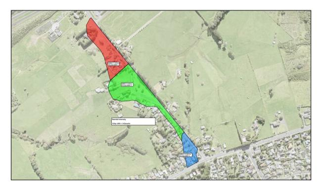
Figure 9: Pre-development catchments for culvert/pipe flows
