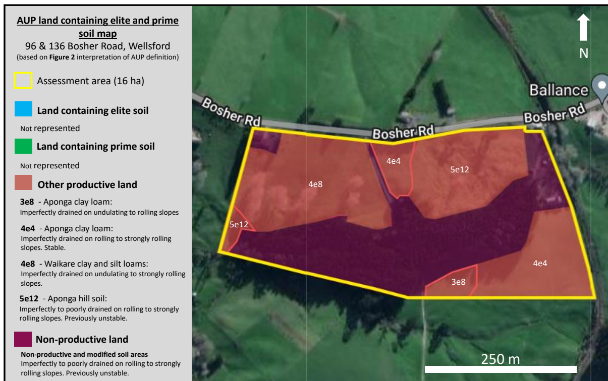
Figure 4. Distribution of soils and LUC units for the assessment area, 96 & 136 Boshier Road. (based on Figure 2 interpretation of AUP definition).
