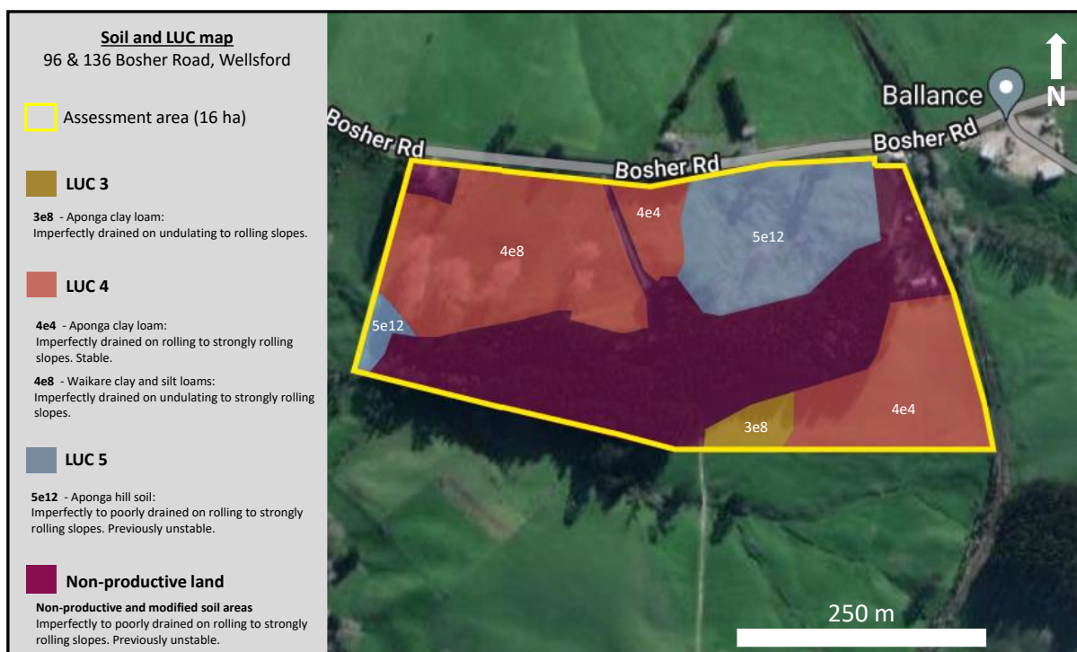
Figure 3. Distribution of soil and LUC map units for the assessment area, 96 & 136 Boshier Road.
