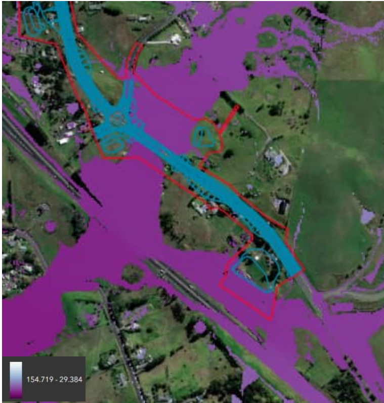
Figure 18-2: NOR13 East Coast Rd upgrade 1% AEP base case flood extents by SH1
