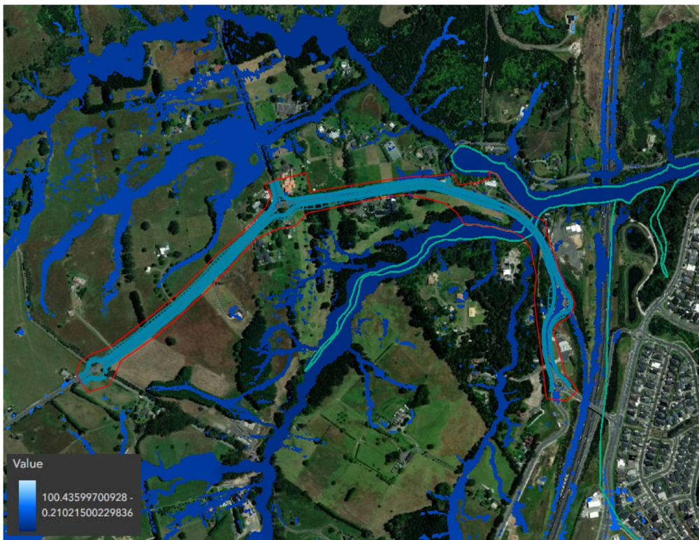
Figure 15-2: NOR10 Wainui Rd upgrade 1% AEP future base case flood extent
