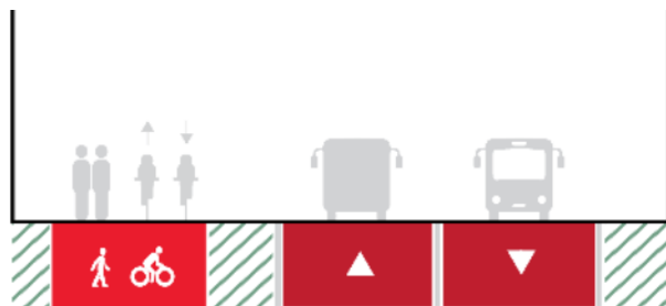
Figure 6-6: Typical Cross Section – Rapid Transit Corridor alongside ASH at Taupaki Road (shared path will re-join Rapid Transit Corridor at Boord Crescent)
