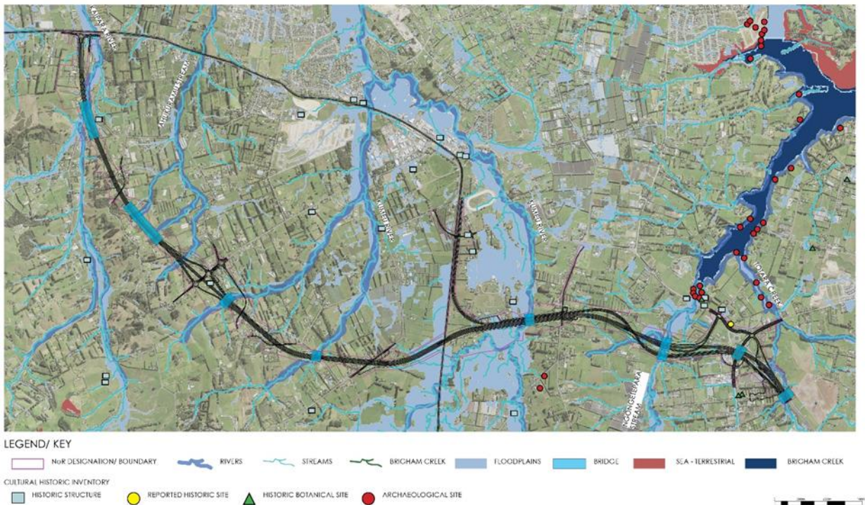
NOR S1 - ALTERNATE SH + BRIGHAM CREEK INTERCHANGE : ECOLOGY, HYDROLOGY AND CULTURAL HERITAGE SITES
