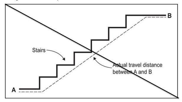
Figure H8.6.18.4 Stair plan distance measurement
