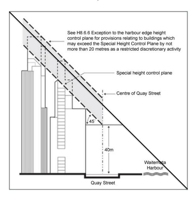
Figure H8.6.6.2 Harbour edge height control co-ordinates[Deleted]
