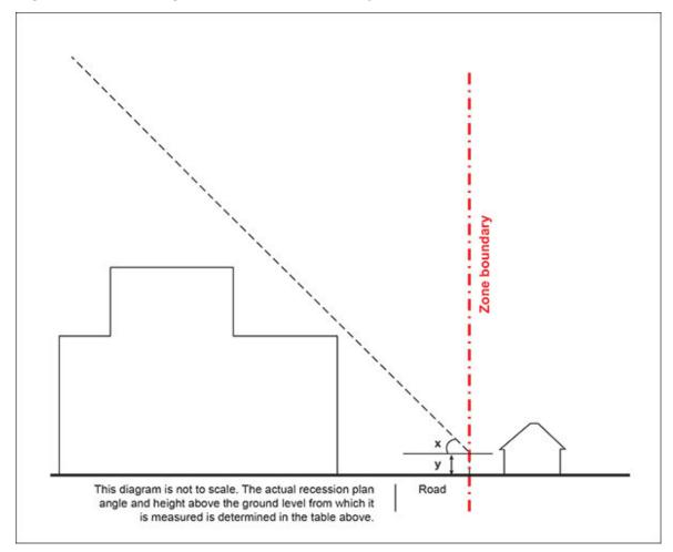
Figure H10.6.2.3 Recession plane indicator for sites adjacent to an open space zone
