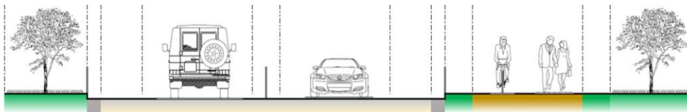
Figure 12-2: Upgrade to Dairy Flat Highway between Dairy Flat and Albany Indicative Design (25m unconstrained cross section)
