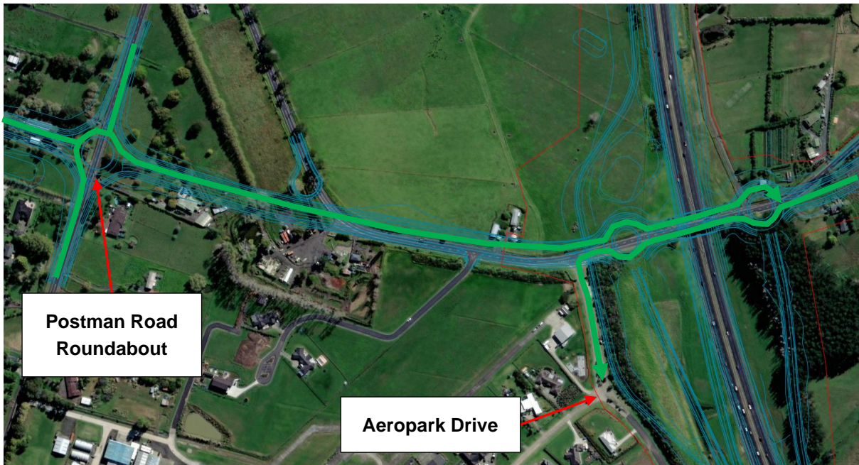
Figure 7-8: SH1 Improvements at Wilks Road Interchange – Aeropark Drive Access – Entry Movements
