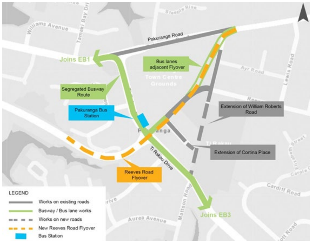
Figure 1 Overview of EB2
