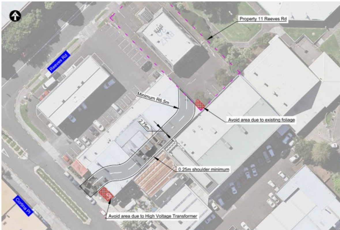
Figure 7.11 Reeves Road temporary access during construction
