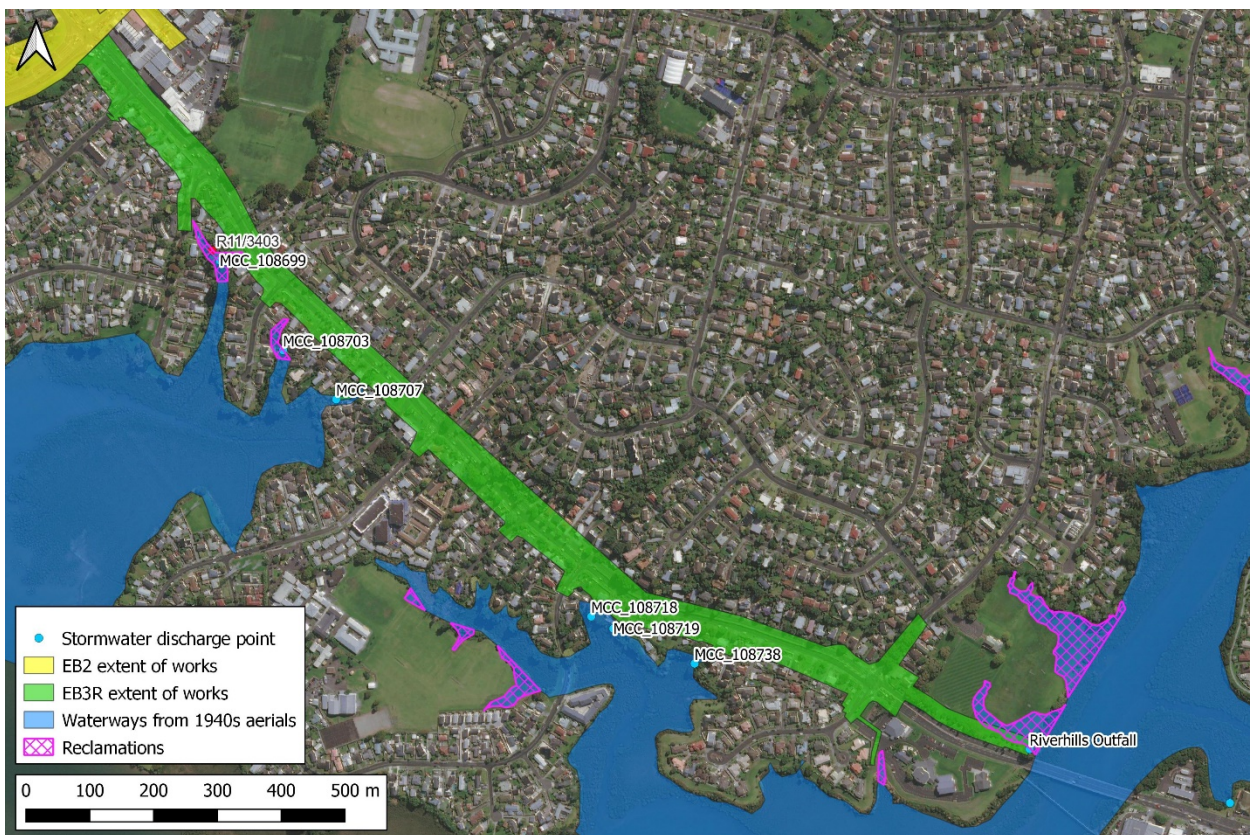
Figure 14. EB3R showing areas where silting or reclamation has obscured inlets and proposed stormwater discharge points.
