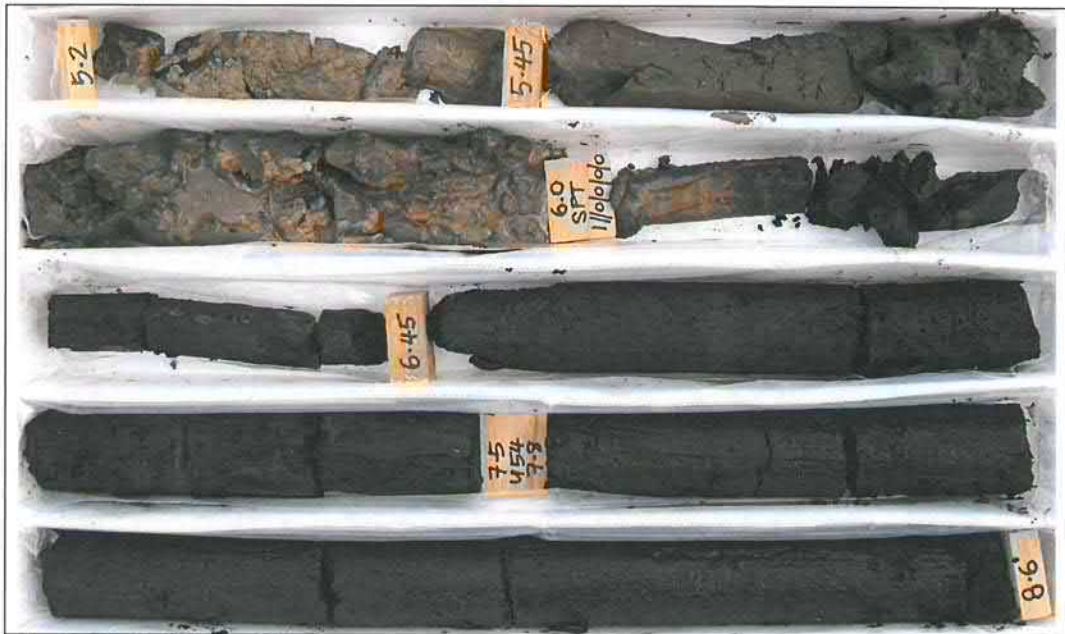
Box 2. - Depth: 5.20m to 8.60m.
