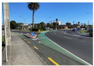
Figure 3-6: Station Road / Wyllie Road intersection with left turn slip lane into Wyllie Road
