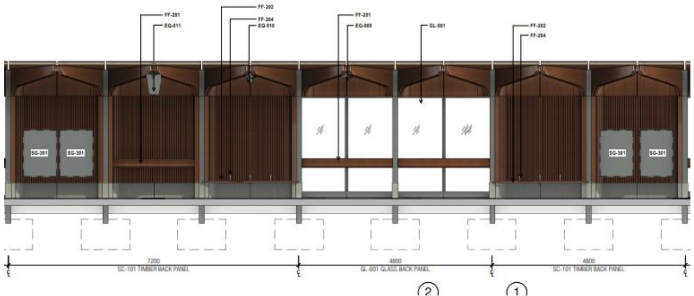
Figure 4-4 Exert of the Front Elevation of East Bound Platform - Pakuranga Bus Station
