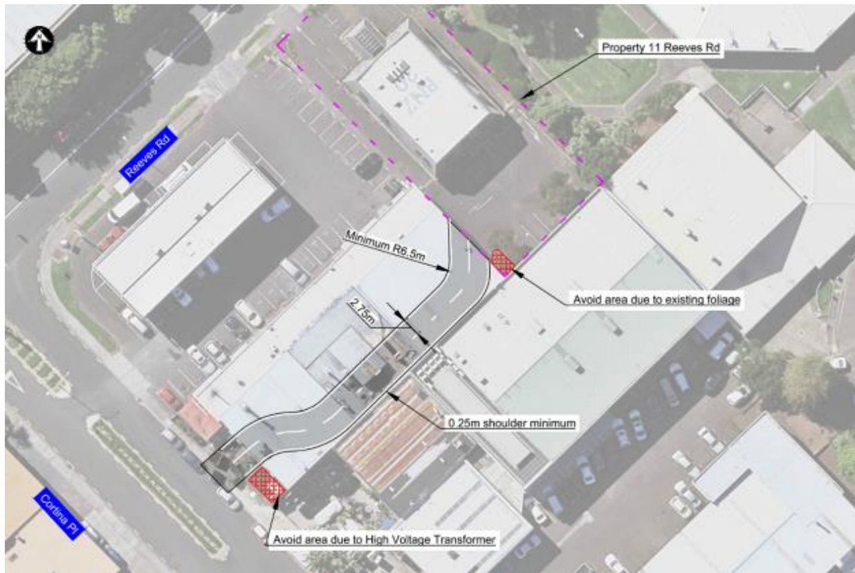
Figure 4-19 Construction Access for 11 Reeves Road
