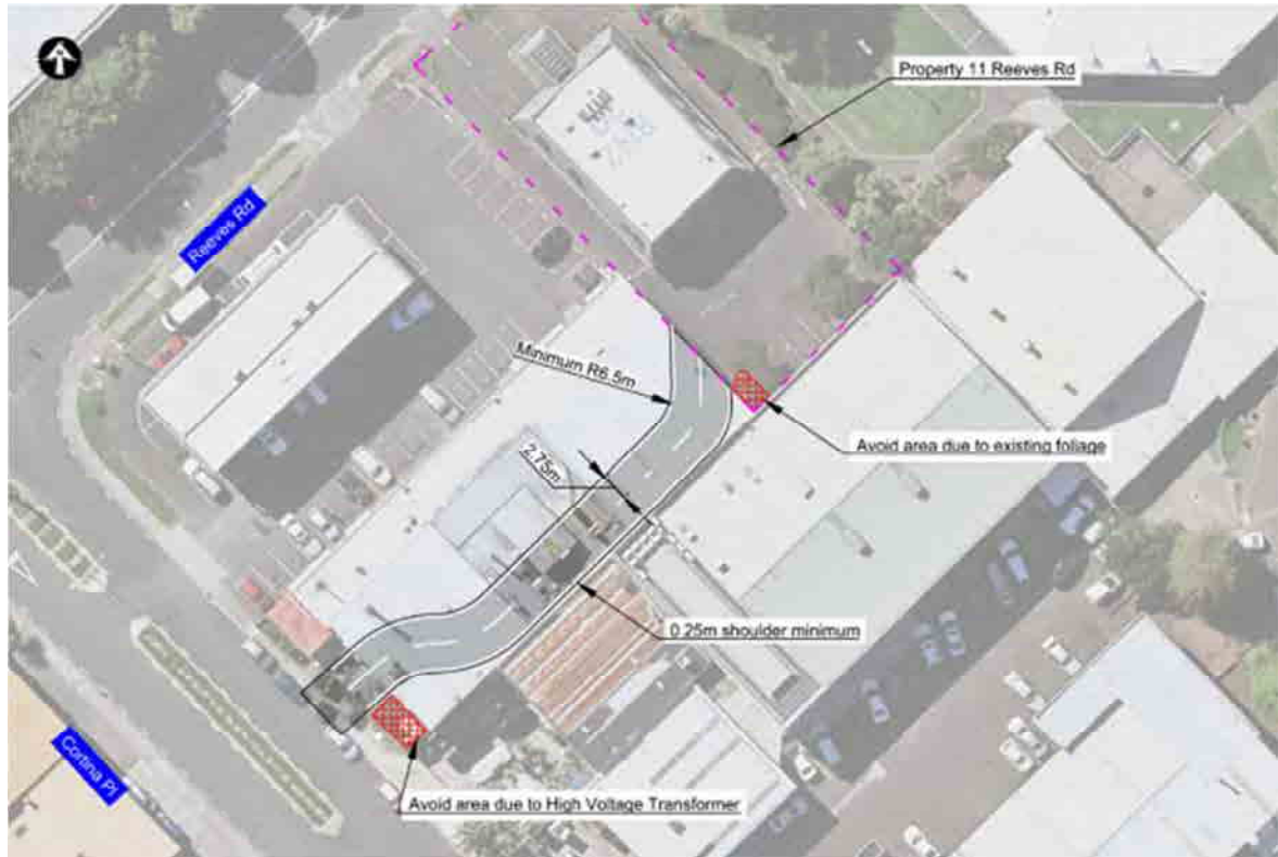
Figure 77: 11 Reeves Rd temporary access during construction
