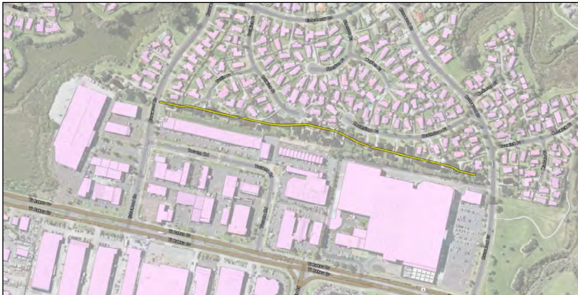
Figure 9-6 Noise barrier that is 2.4m in height to be constructed within Burswood (Yellow Line)
