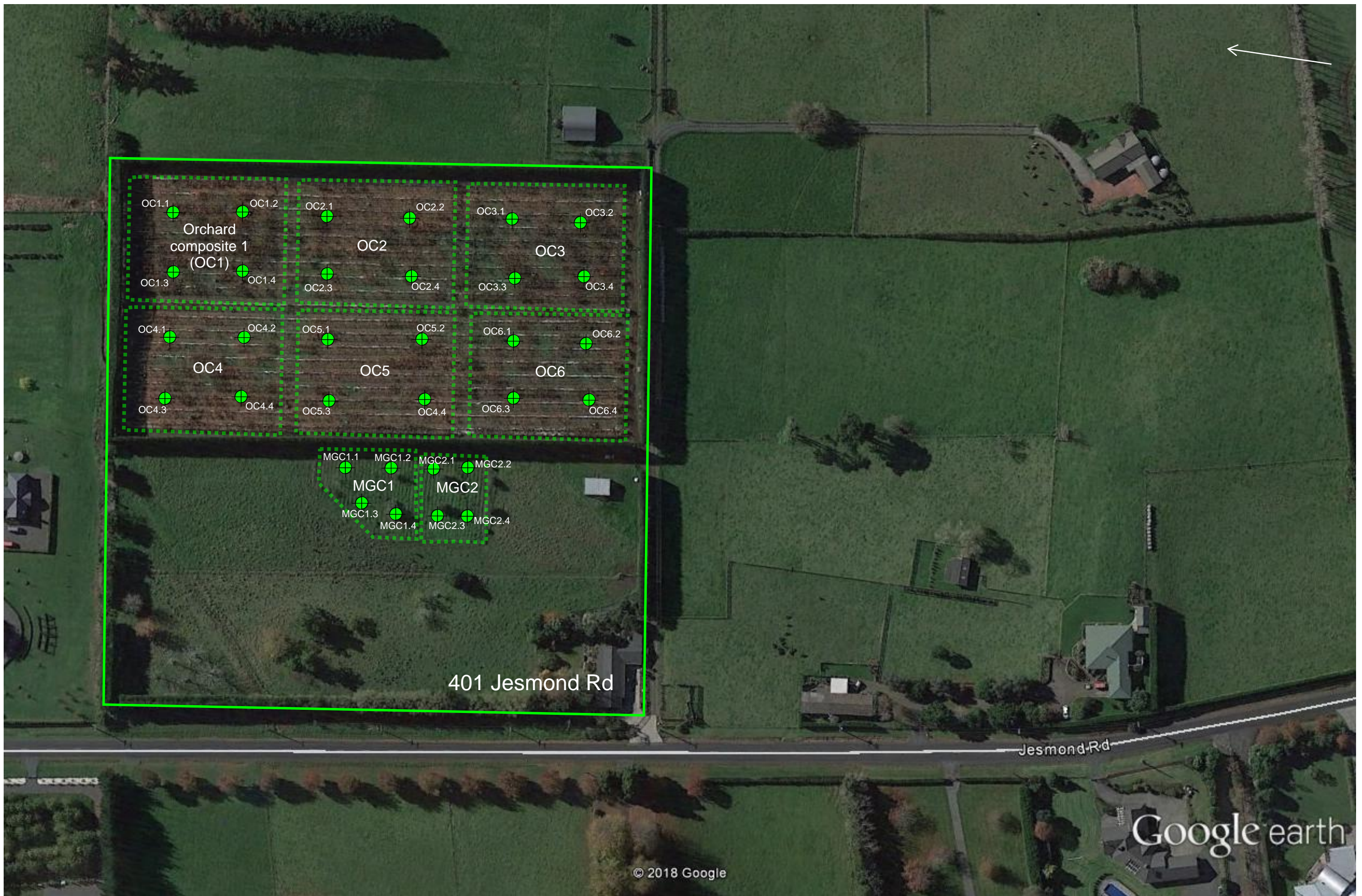
Soil Sample Location Plan - Contamination Assessment , 401 Jesmond Road (1st and 2nd August 2018)
