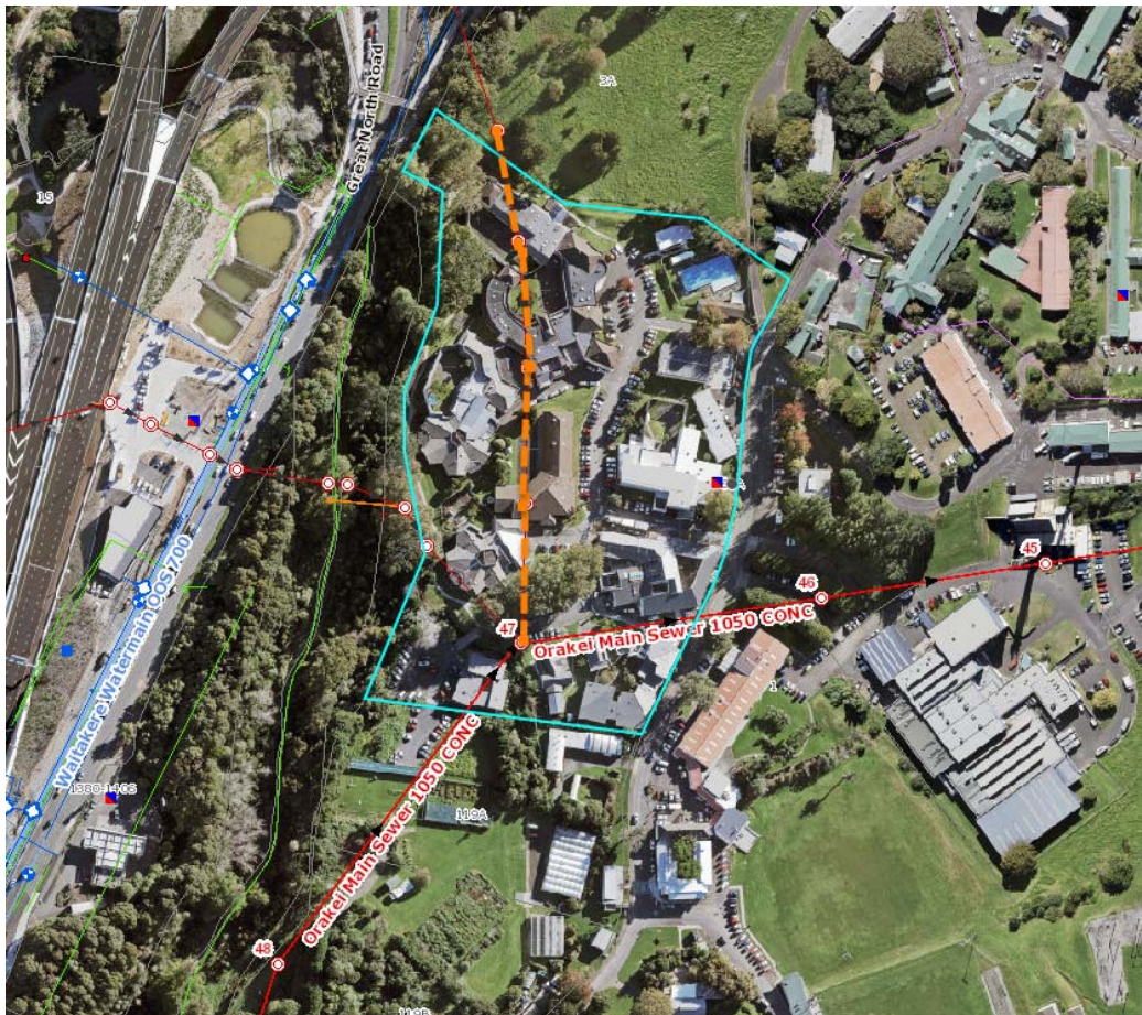
375mm SS network with possible constraints (highlighted in orange) that requires asset investigation.
