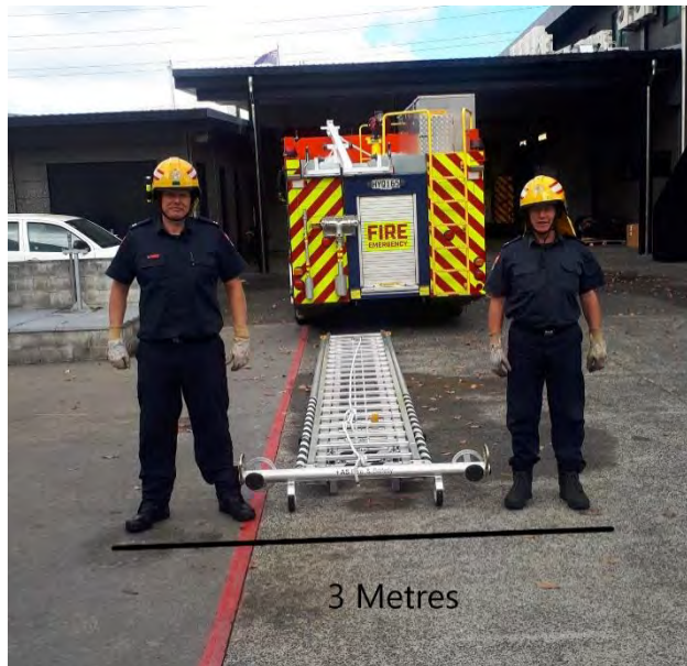
Figure 2: Width of Angus 464 Rescue Ladder with crew
