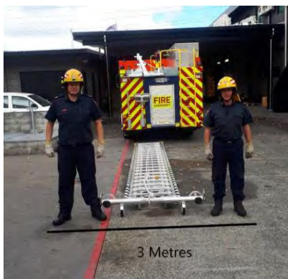
Photos 28 & 29: Width and turning arc of Angus 464 Rescue Ladder with Crew (Source: FENZ)
