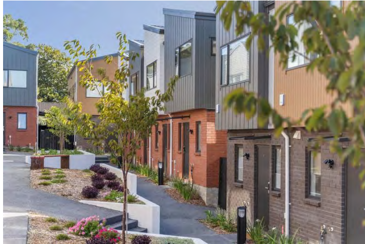
Photograph 38: Landscaped buffers (minimum m) between dwelling and pedestrian access routes as well as additional communal area planting that contributes positively to the amenity of the approach to the dwellings
