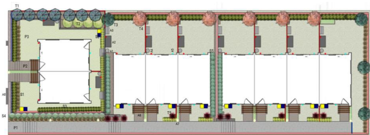
Pedestrian only access, 1.5m wide pedestrian path, 45m length serving 7 Units with front courtyards. Path has steps and ramps, boundary retaining walls and dead-end single entry/exit
