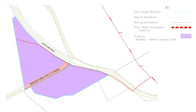
Figure 8 - Indicative Plan Change Wastewater Layout
