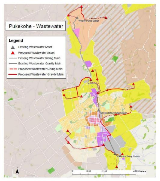
Figure 7 Pukekohe Paerata Structure Plan Wastewater Assets (Source Structure Plan)
