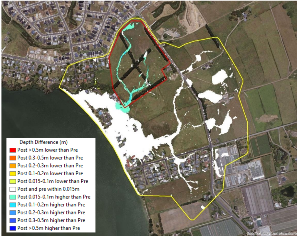
FIGURE 26: 1% AEP depth difference, ED + MPD minus ED flood model scenarios (no SLR).
