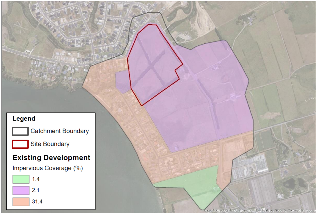
FIGURE 30: ED scenario model extent and imperviousness.
