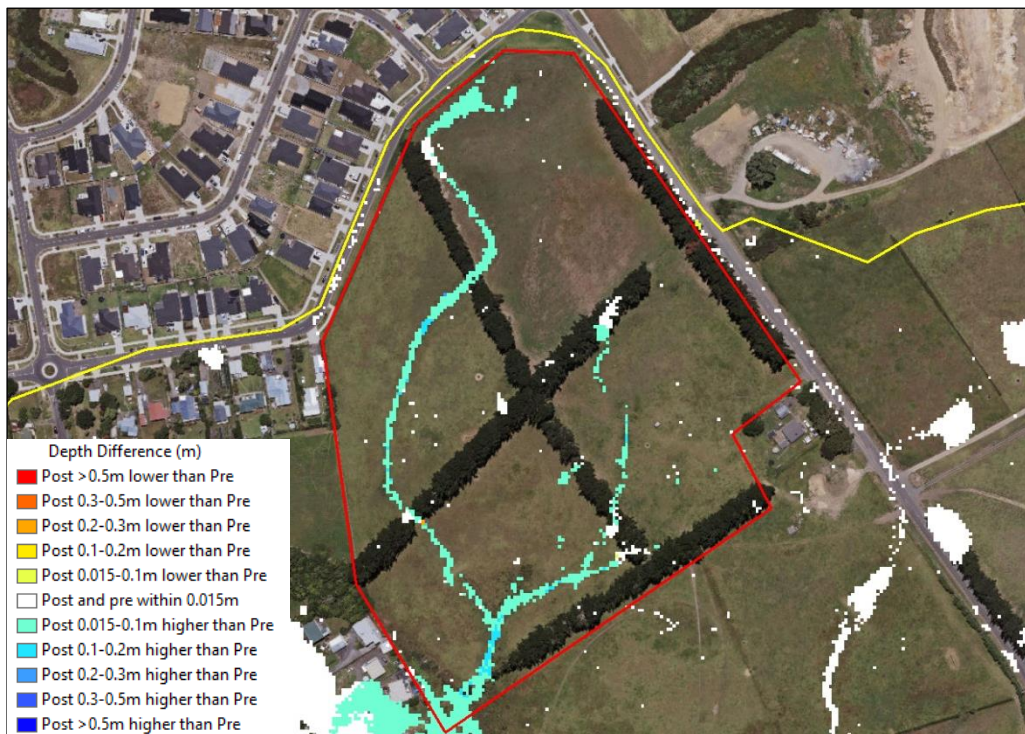
FIGURE 20: 10% AEP on site depth difference, ED + MPD minus ED flood model scenarios (1 m SLR).
