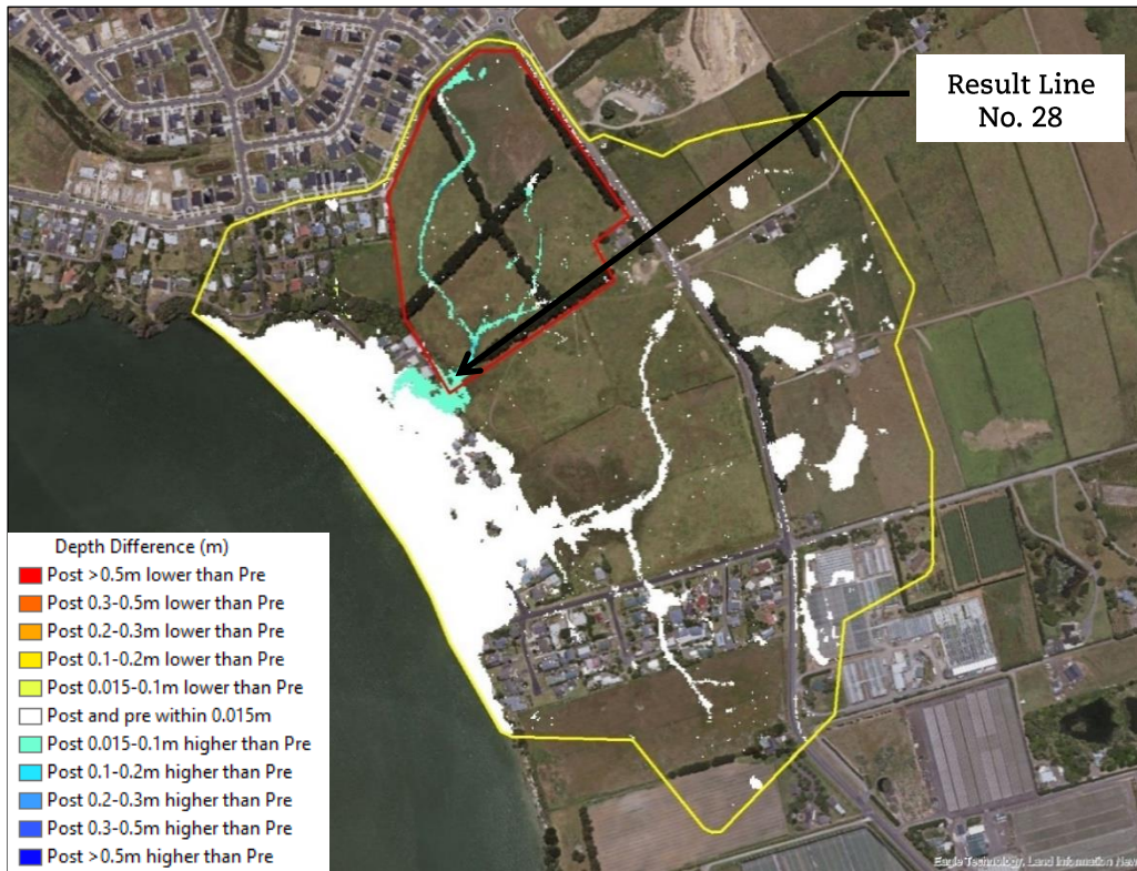
FIGURE 19: 10% AEP catchment wide depth difference, ED + MPD minus ED flood model scenarios (1 m SLR).
