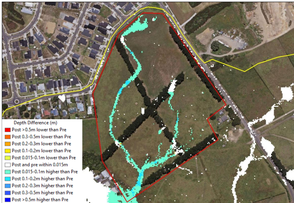
FIGURE 18: 1% AEP on site depth difference, ED + MPD minus ED flood model scenario (1 m SLR).
