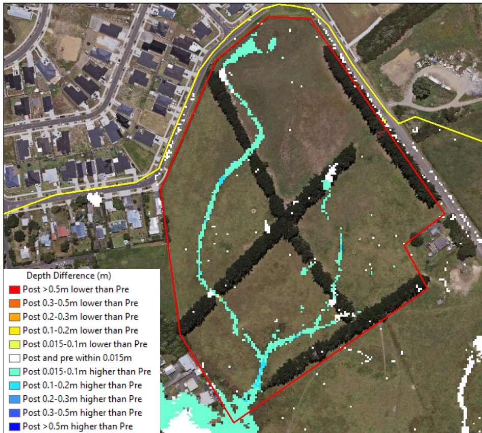
FIGURE 26: 10% AEP on site depth difference, ED + MPD on-site minus ED flood model scenarios (no SLR).
