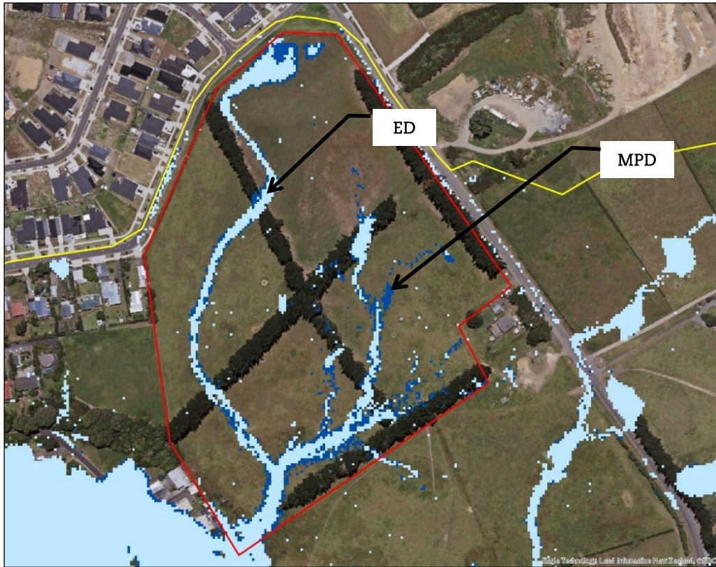
FIGURE 21: 1% AEP ED and MPD scenario flood extents (1 m SLR).
