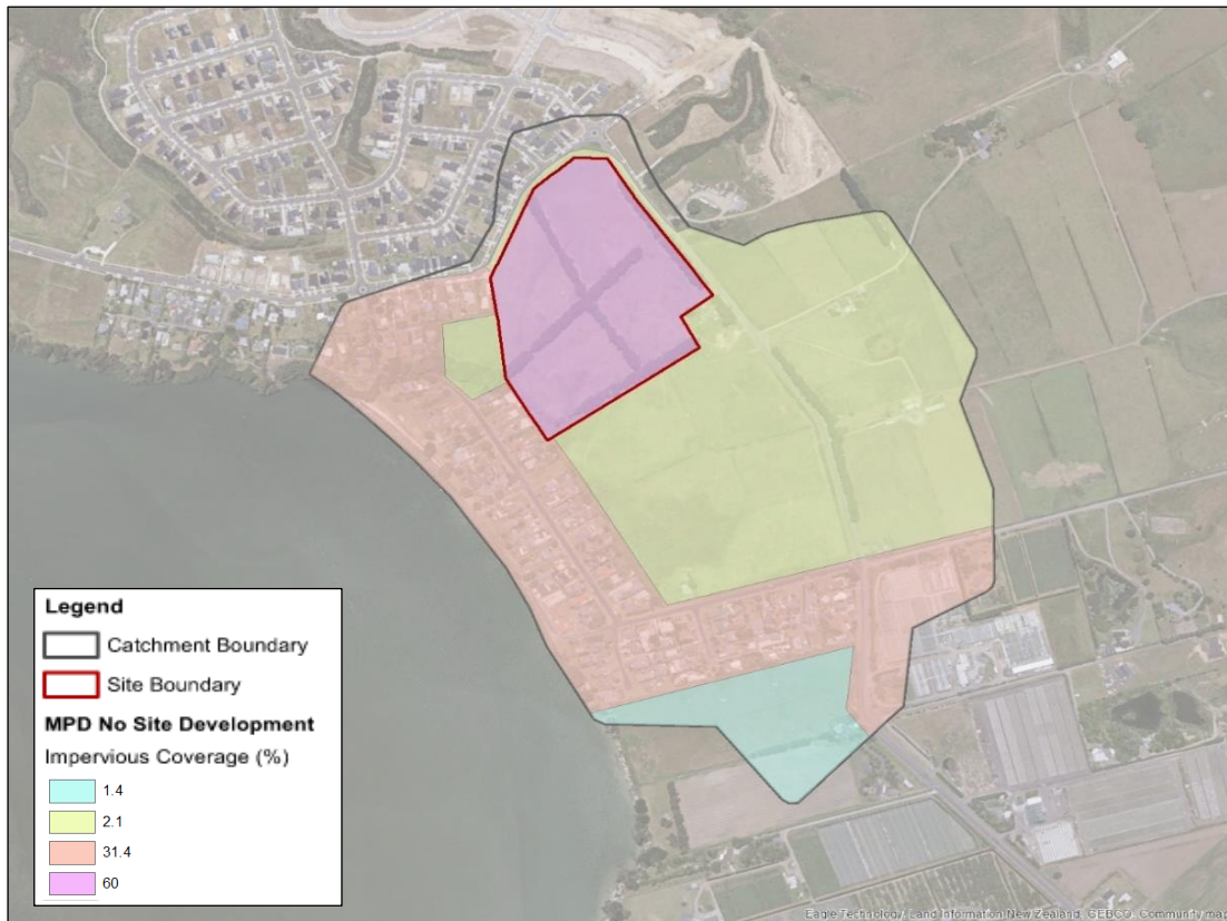
FIGURE 32: ED+MPD site scenario model extent and imperviousness.
