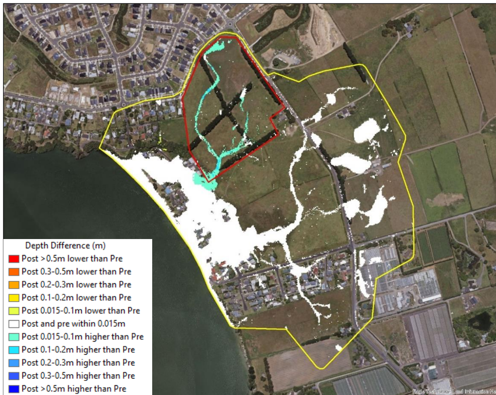
FIGURE 23: 1% AEP catchment wide depth difference, ED + MPD on-site minus ED flood model scenarios (no SLR).
