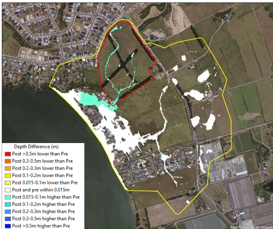
FIGURE 25: 10% AEP catchment wide depth difference, ED + MPD on-site minus ED flood model scenarios (no SLR).
