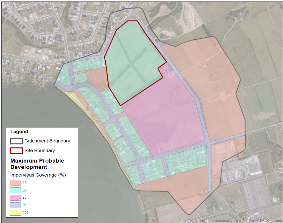
FIGURE 31: MPD scenario model extent and imperviousness.
