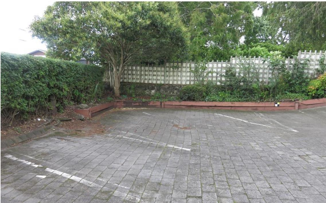
Figure 30: Paved car parking area in the front yard. The street boundary hedge conceals a rubble basalt stone wall, and a basalt wall also runs along the southern boundary to 151 Gillies Ave, below the trellis fence.
