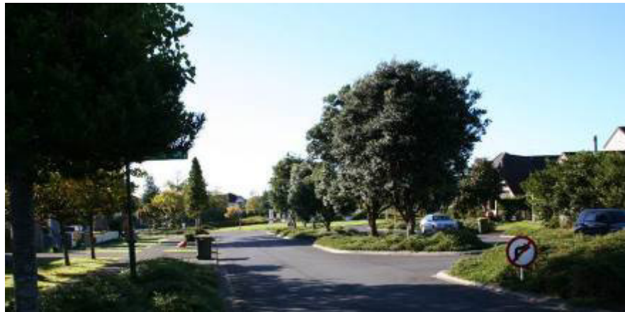
Photograph 26: This boulevard in Te Atatu demonstrates how a broad, well planted median can minimise the dominance of the carriageway and contribute considerably to the amenity of the road corridor.
