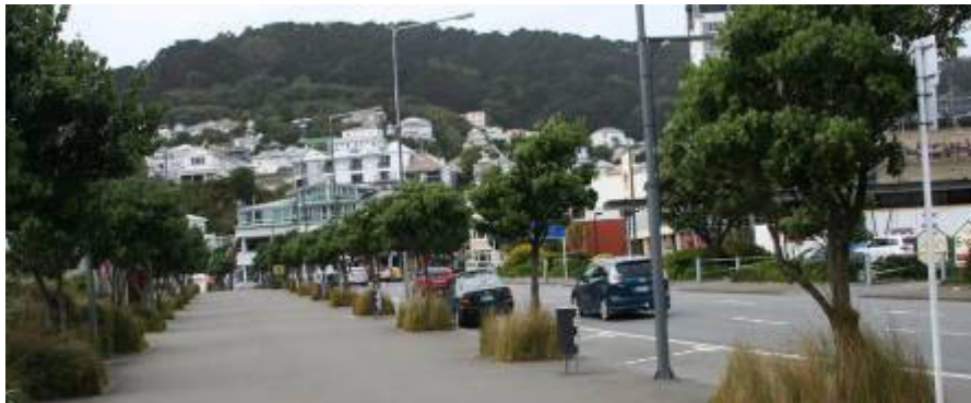
Photograph 28: This generous roadside path employs street trees and related infiltration beds as a device to physically and visually separate the non-vehicular space from the road.
