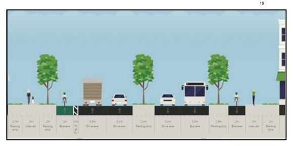
FIGURE 9: 32M TYPICAL ARTERIAL CROSS SECTION
