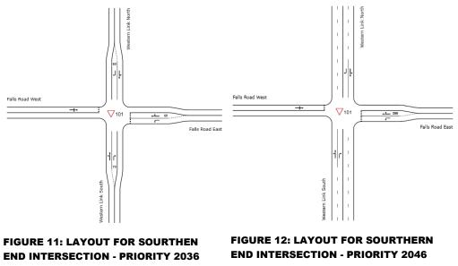
The proposed layouts for 2036 and 2046 for Western Link and Falls Road intersection with priority control is shown in figures below:
