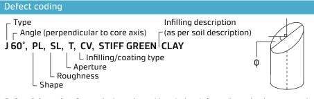
**Defect Orientation:** for vertical unoriented boreholes defect orientation is measured normal to core axis e.g horizontal =  $0^{\circ}$  (see diagram). For angled boreholes defect orientation is measured relative to core axis e.g parallel to core axis = 0°.
