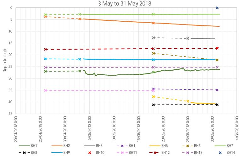
Notes: Solid Line = Groundwater level based on Sonlist Levelogger 'continuous' monitoring (one reading every 5 minutes).
