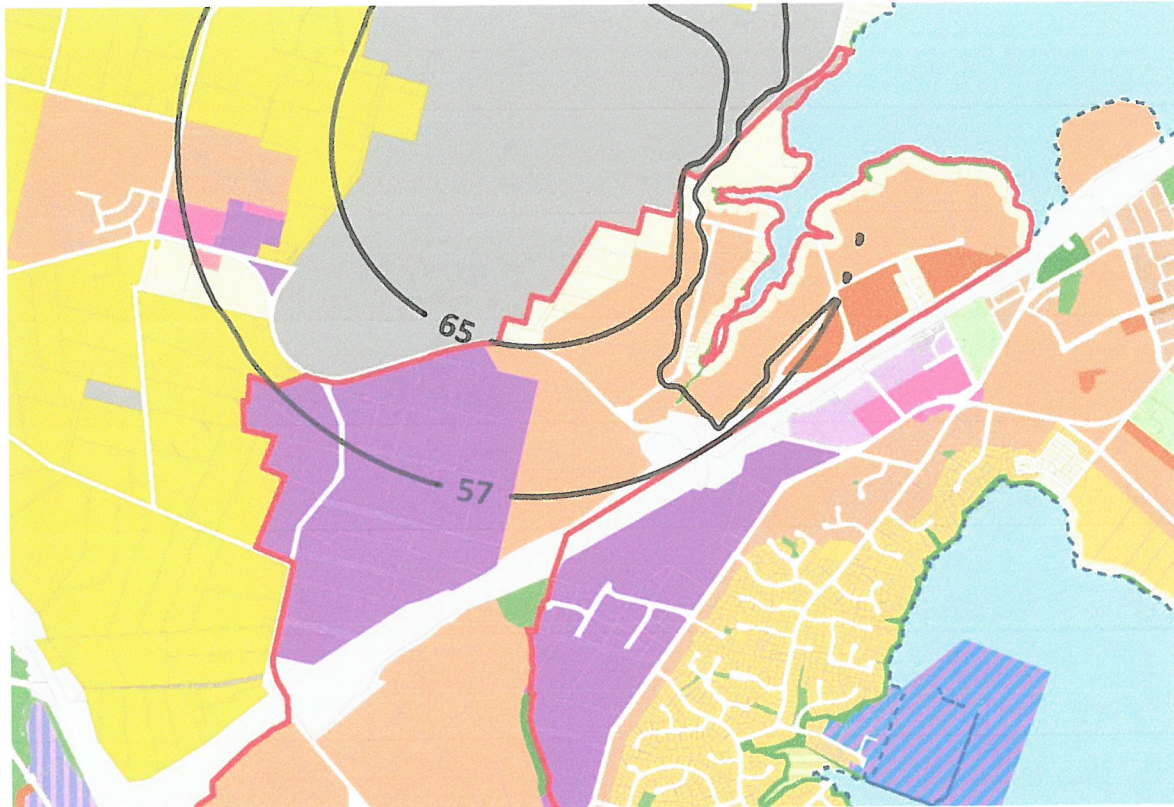
Figure 13 Map showing LAeq(24 hr) 57 dB and 65 dB contours for cumulative noise from engine testing of the B757, C130 and P3 aircraft conducted at Whenuapai Airbase over a 'worse case' seven day rolling time period recorded during the 60 day survey of engine testing conducted in 2016.
