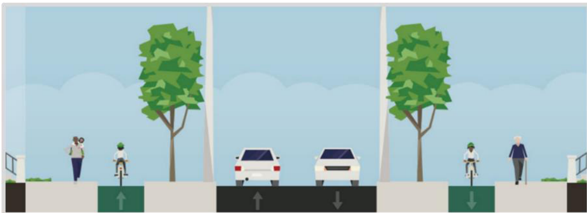
Figure 18: Collector Road cross section (20m)
