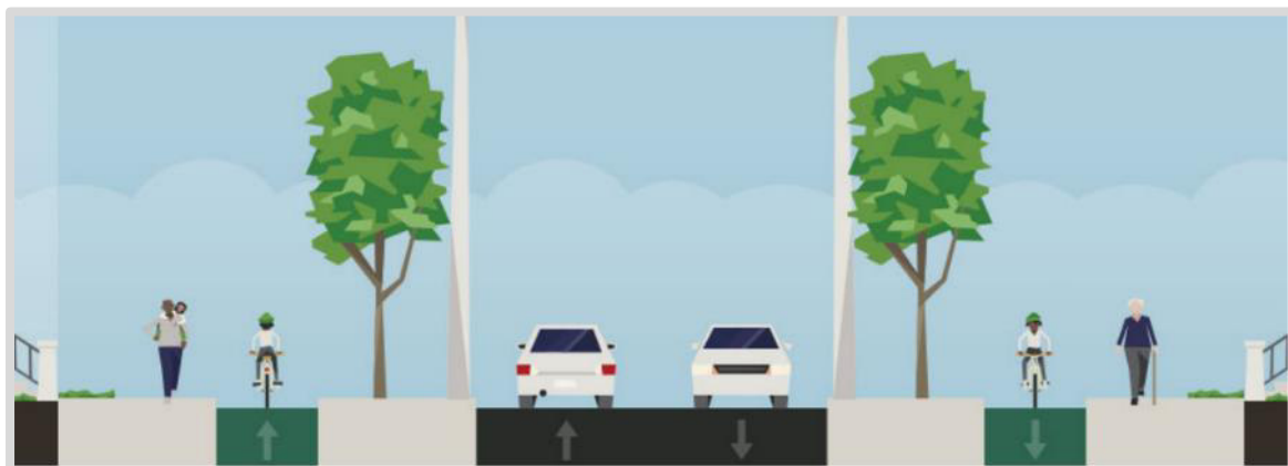
Figure 11: SGA ITA Urban Collector Road Indicative Cross Section (21m)
