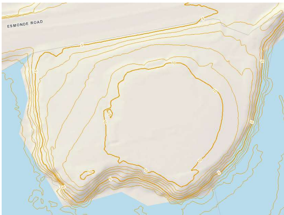
Figure 3-1: Contours showing maximum cliff height of 10m at steepest part of slope with remaining height ranging from 5m to 8m (Source: AC GIS viewer)
