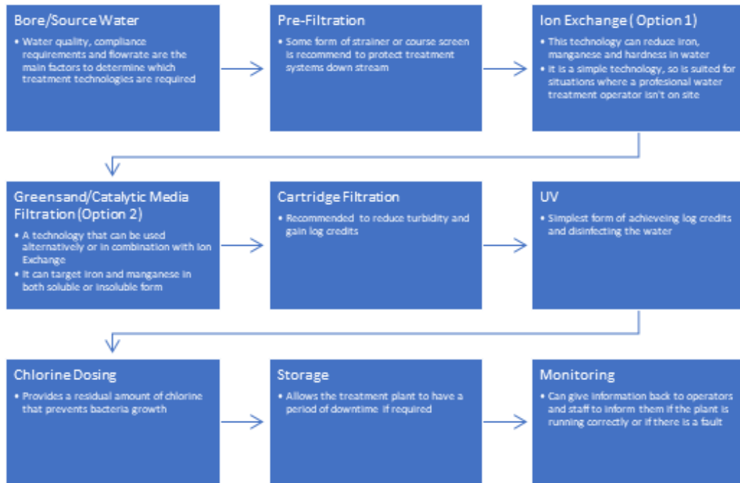
Figure 3: Proposed Water Treatment Process Flow Diagram
