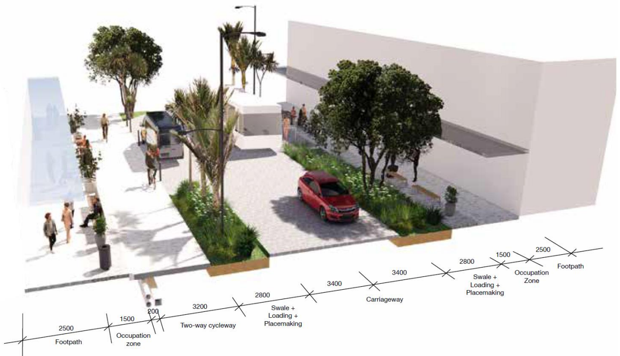
Figure 13. Street Cross-section: Primary Collector (Village Centre)
