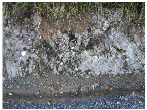
Photo 2: Moderately strong siltstone with minor sandstone exposed adjacent to McNicol Road
