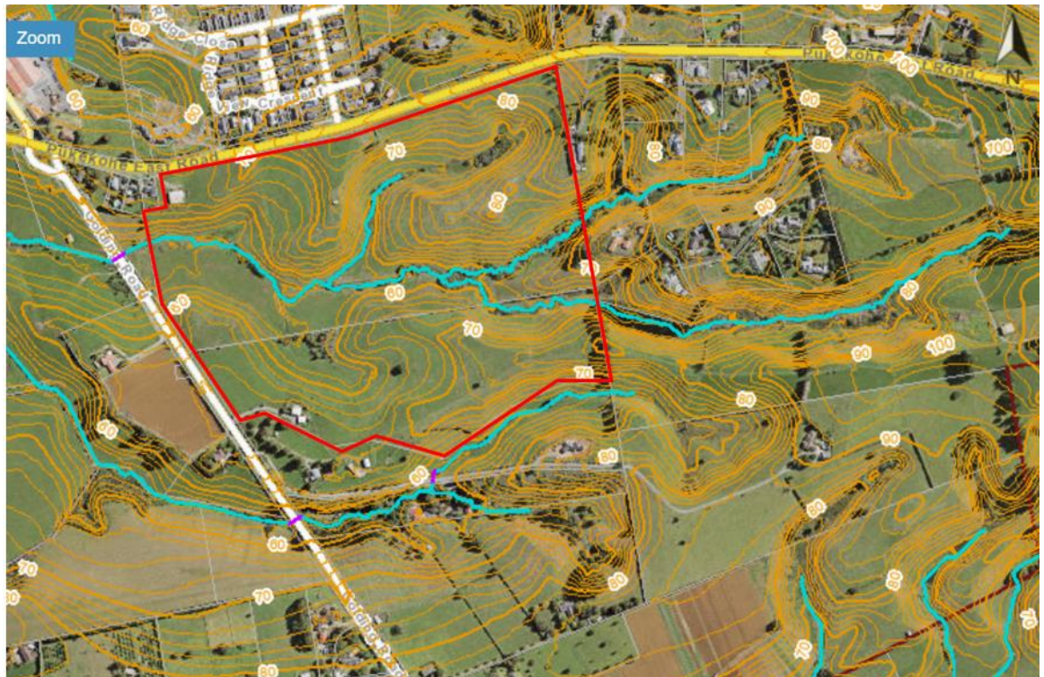
Figure 18. Aerial plan with contours showing the permanent streams (blue lines) in the Plan Change Area, which is outlined in red (source: Auckland Council Geomaps)
