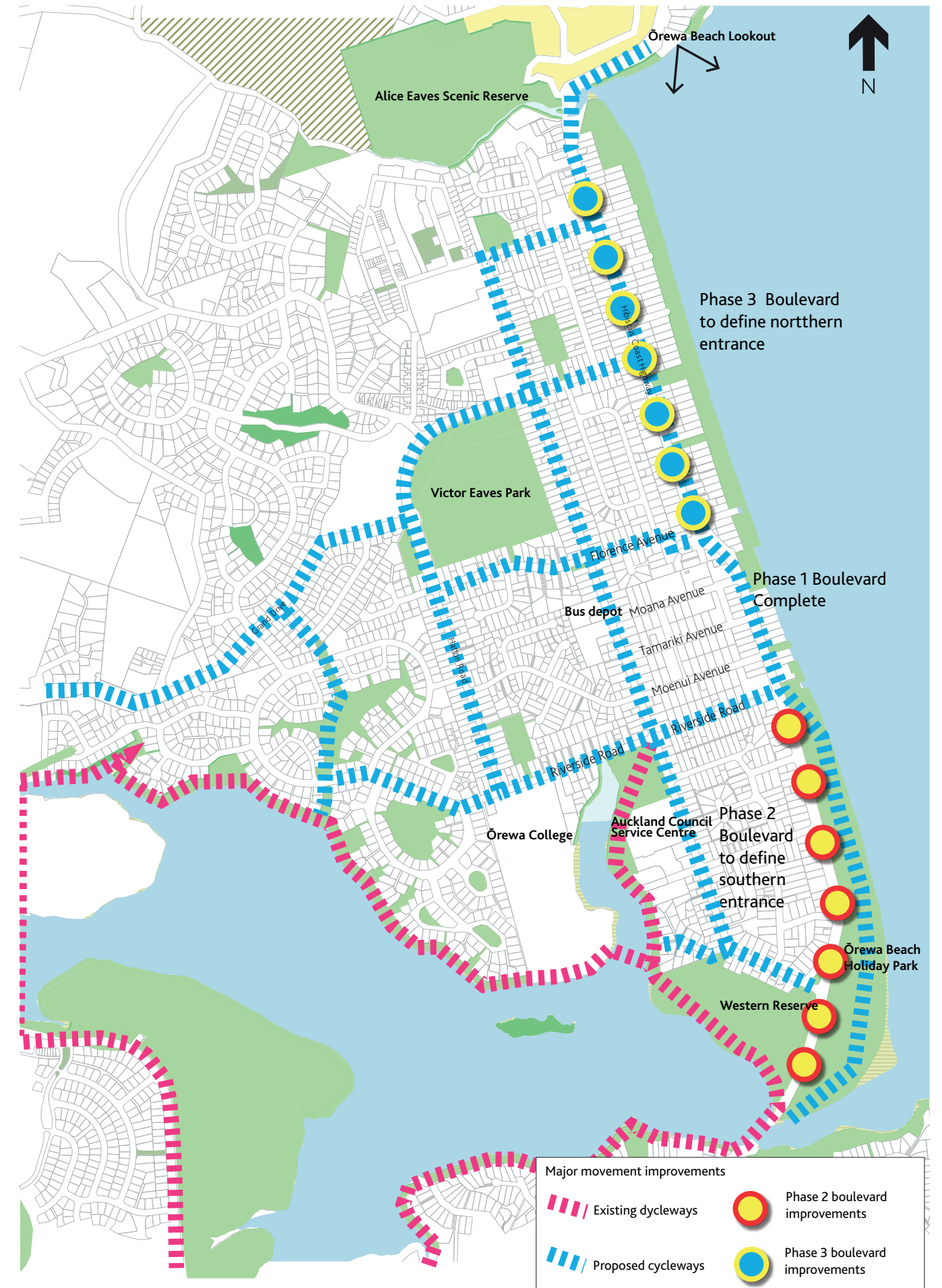
Existing and proposed cycleways to establish a better network for cycling around the town centre.
