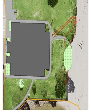
Long term, proposed re-direction of entry and landing onto the beach and extension of dune cell immediately east of the car park.
