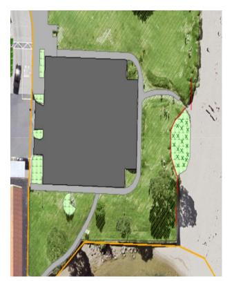
Temporary silt fencing and bolstering of existing dune cell to happen in the short term.
