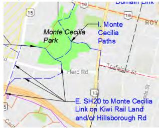
This is not an easy connection, but given the high use of the SH20 Cycleway, it is a very strategic route. The most direct connection is to create a shared path down the eastern side of Hillsborough Rd. The has been investigated and would require purchasing a small sliver of property near the intersection of Hillsborough and Haughey Ave before connecting with the park at Delargey Ave.
